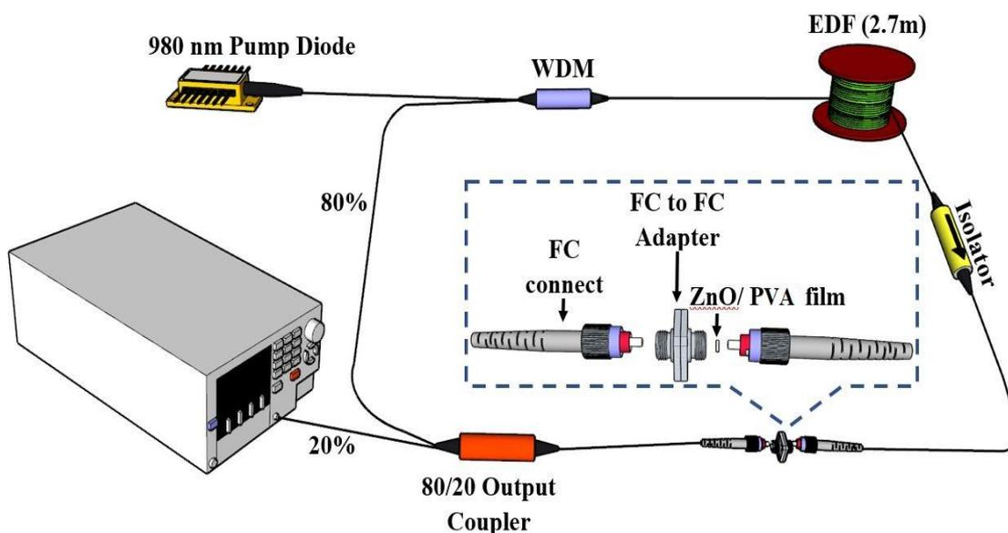
Fig. 3. Erbium-doped fiber laser set up the cavity
