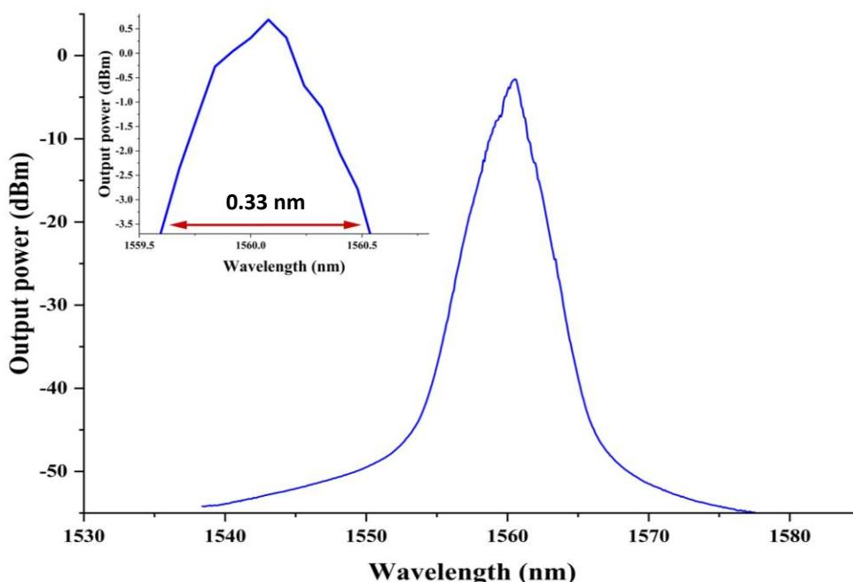
Fig. 4. Optical spectrum of the ZnO nanoparticles-PVA SA based Q-switched EDFL at 157.01 mW
