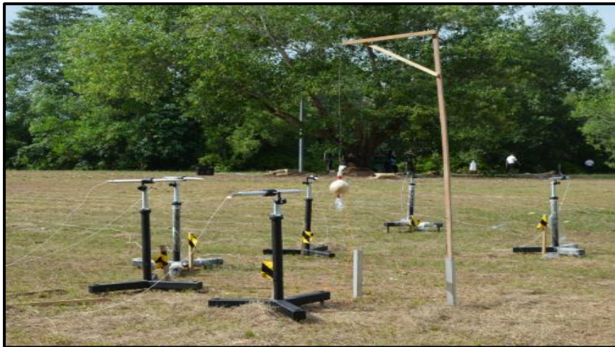
Fig. 3. Field blast test set up [3]
