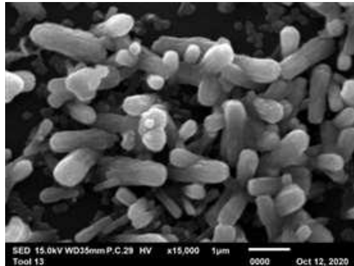
Fig. 3. SEM of ZnO in crystallization shapes
