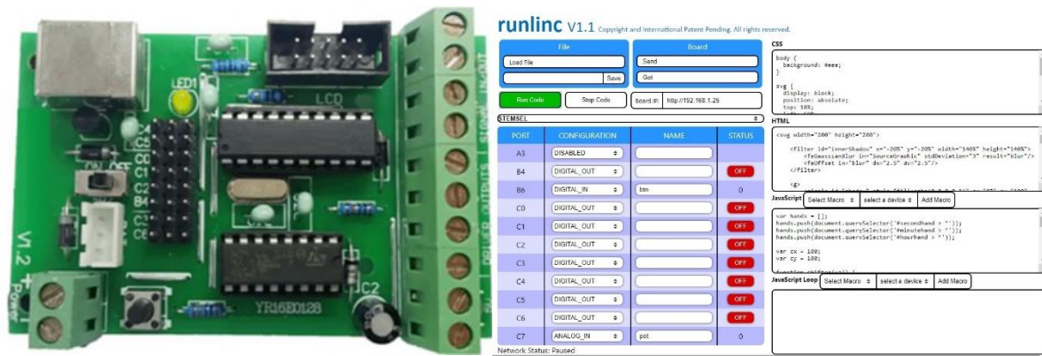
Fig. 4. STEMSEL module and Typical Runlinc IDE webpage
