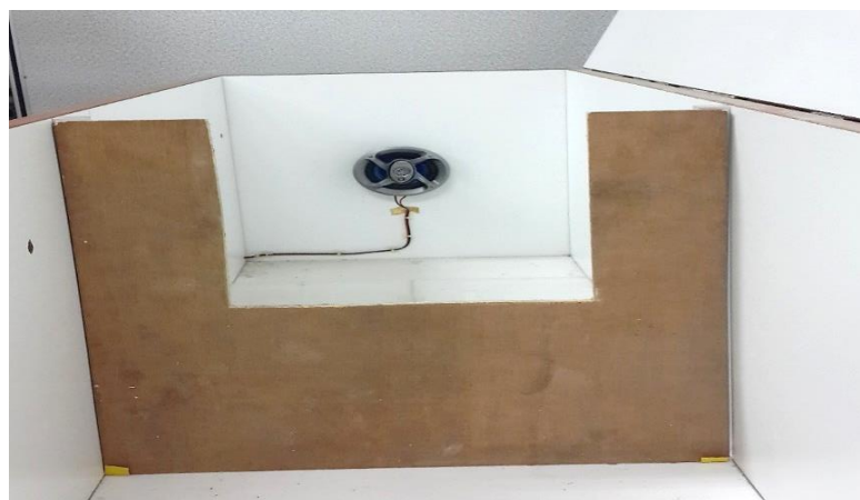
Fig. 7. Inside of noise effect system chamber with no partition
