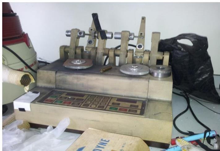
**Fig. 1.** Pin-on-disc wear machine
