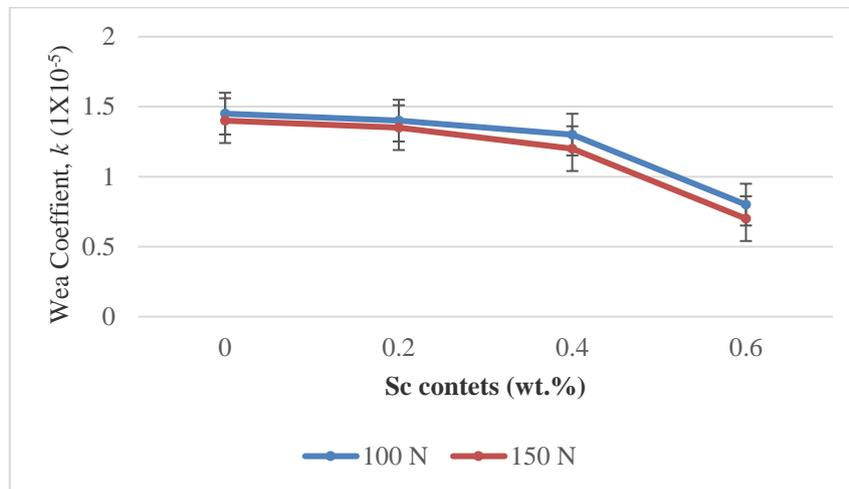
**Fig. 5.** Wear coefficient of Al-7Si with different Sc contents conducted at 1000 m distance
