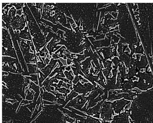
**Fig. 3.** FESEM morphology of Al-Si alloy reinforced with 0.8 wt.% Sc with 500 X magnification
