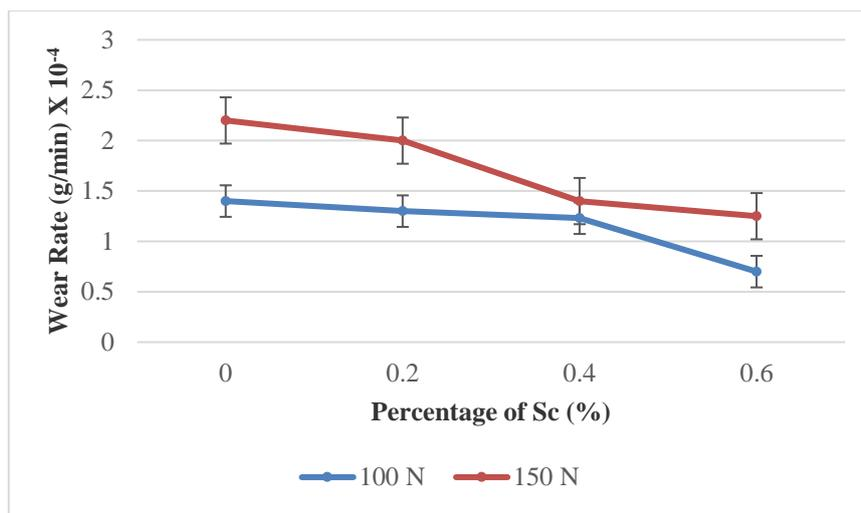
**Fig. 6.** Wear rate (g/min) of Al-Si-Sc composite alloy in wear test conducted in 1000 m within 1 hour at different loads (N)
