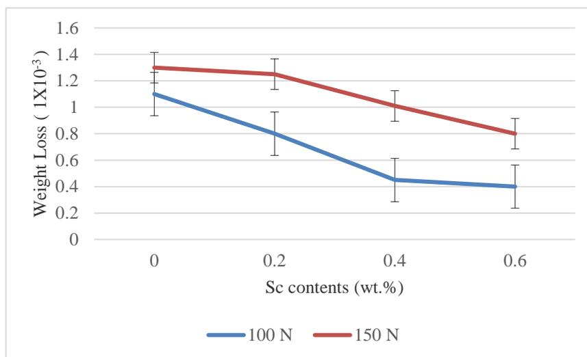
**Fig. 4.** Weight loss (g) of Al-7Si-Sc in wear test conducted at 1000 m distance with different applied loads (N)
