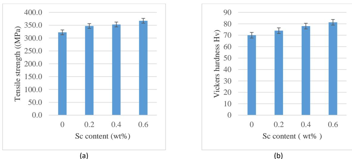
**Fig. 2.** Al-Si alloy reinforced with different Sc contents (a)Tensile strength (MPa) (b) hardness (Hv)
