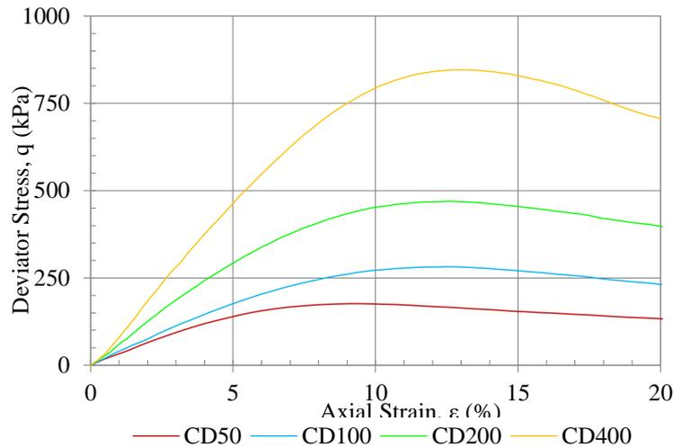
**Fig. 5.** Stress – strain behaviour for CD test
