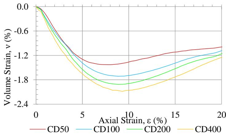
**Fig. 7.** Volumetric strain – axial strain for CD test
