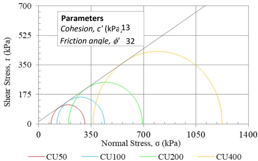
Fig. 4. Mohr-Coulomb failure envelope for CU test
