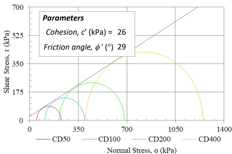
**Fig. 3.** Mohr-Coulomb failure envelope for CD test
