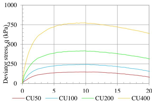
**Fig. 6.** Stress – strain behaviour for CU test
