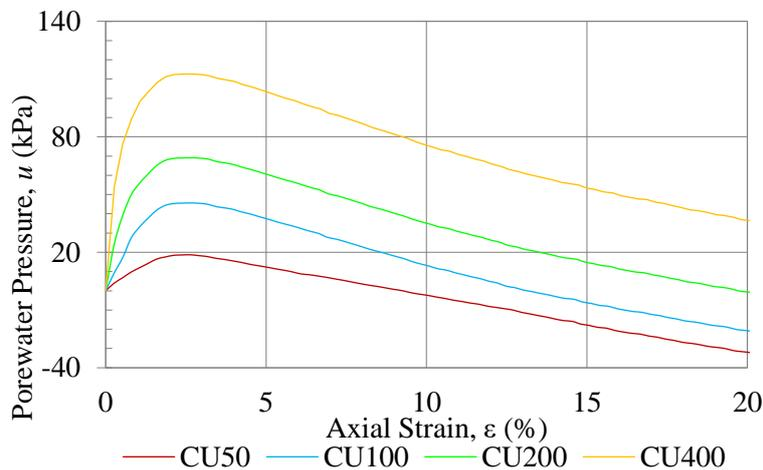
**Fig. 8.** Porewater pressure – axial strain for CU test
