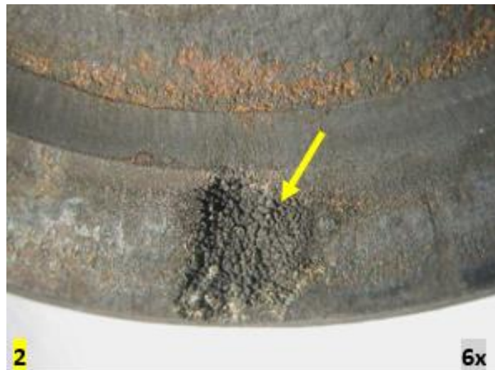
Fig. 4. On the valve seat, carbon
