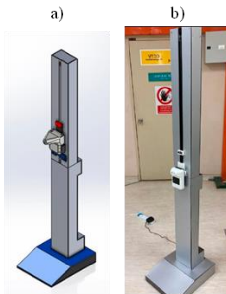
Fig. 1. (a) 3D design Smart Adjustable stand (b) Fabricated Smart Adjustable stand
