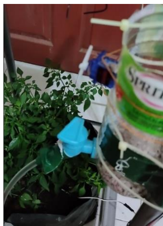
Fig. 6. Servo motor turn on the valve of fertilizer
