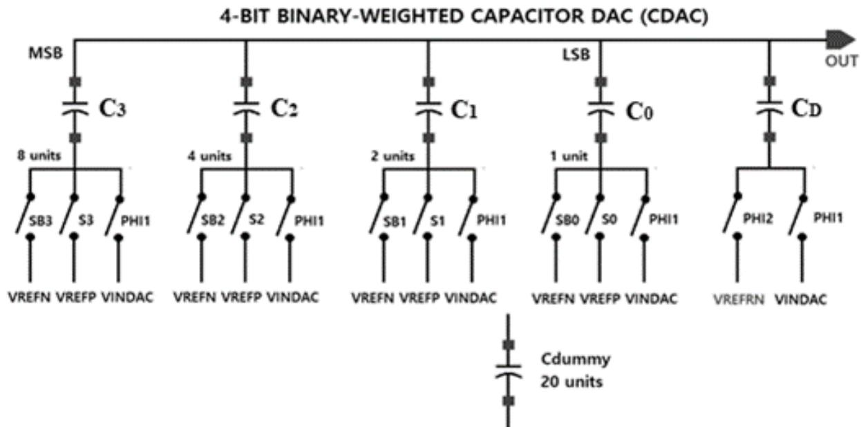
Fig. 3. Schematic Diagram of the 4-bit Capacitor DAC (CDAC)
