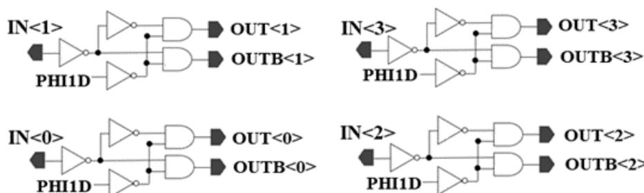
Fig. 2. Schematic Diagram of the 4-bit multiplexer (MUX4)
