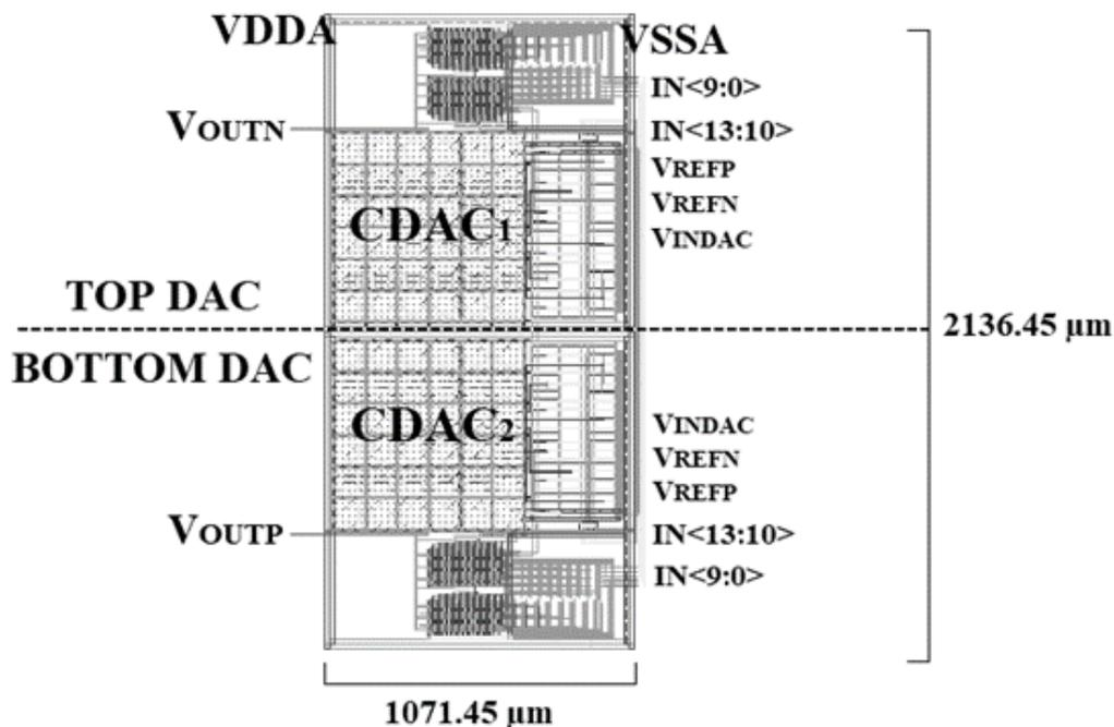
Fig. 7. Layout design of the top-level differential DAC
