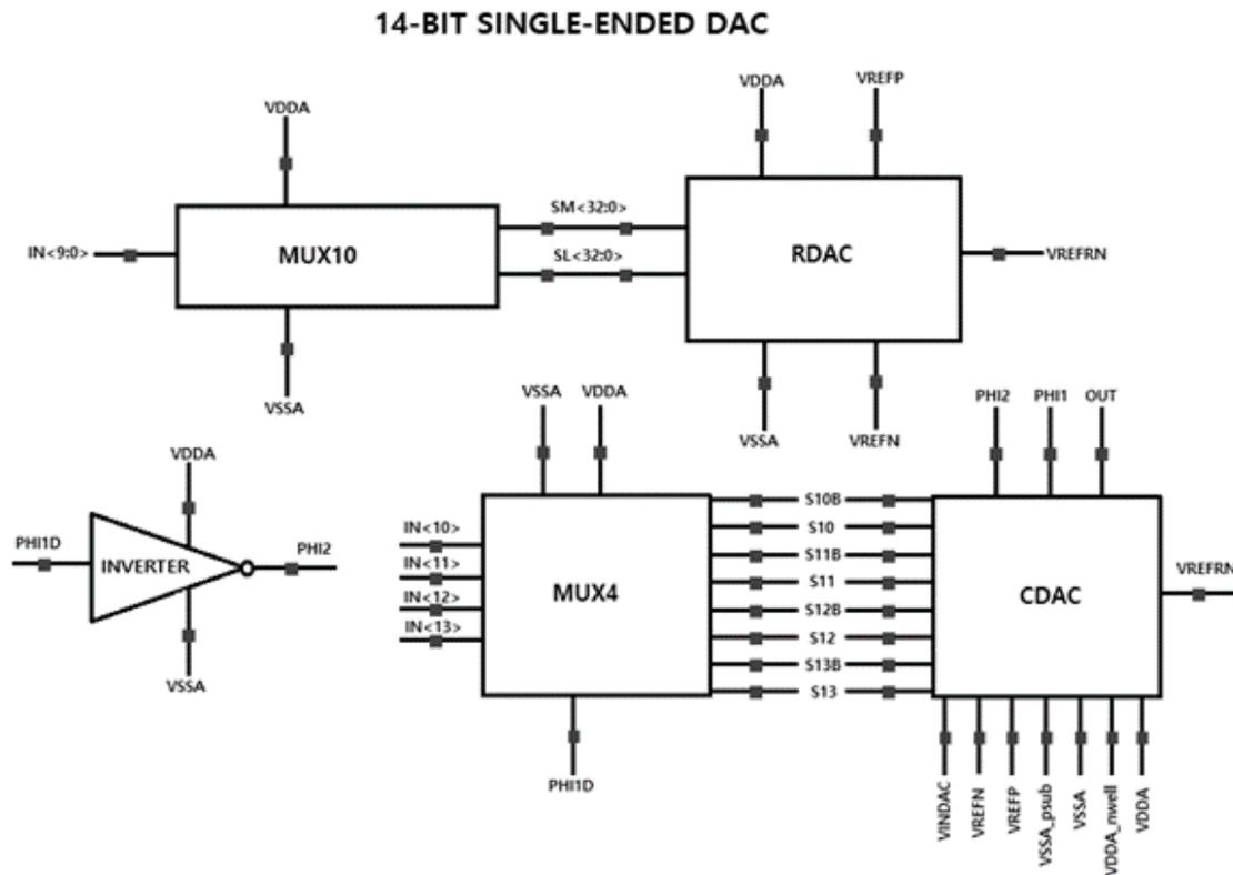
**Fig. 6.** Schematic diagram of the 14-bit single-ended DAC at the top level
