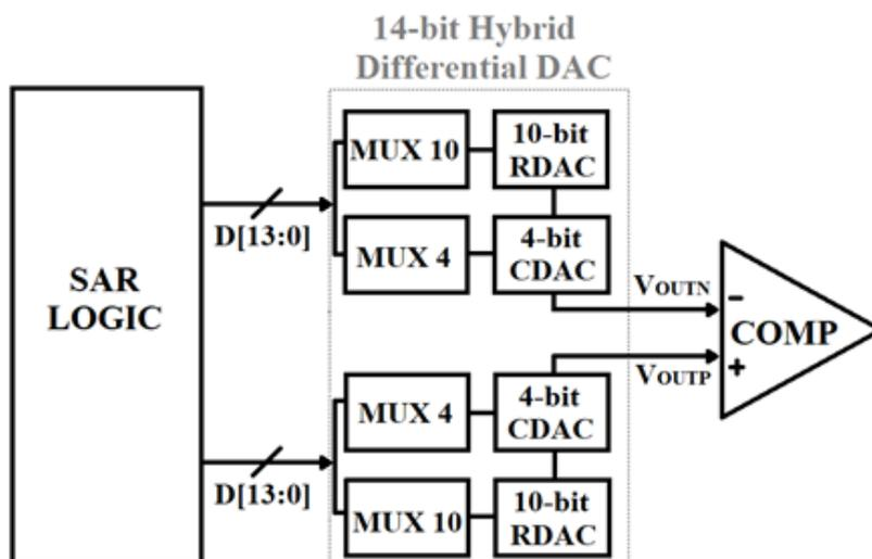
Fig. 1. Block Diagram of the 14-bit single-ended hybrid DAC
