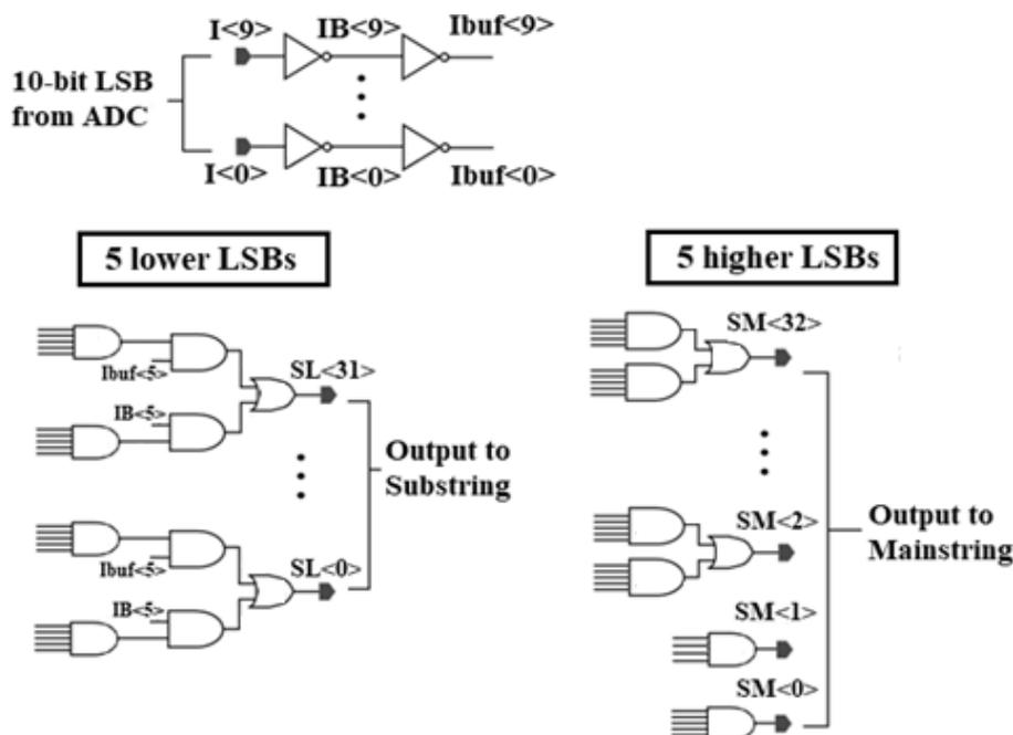
Fig. 4. Schematic Diagram of the 10-bit multiplexer (MUX10)
