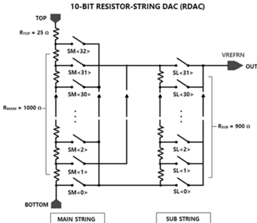
**Fig. 5.** Schematic Diagram of the 10-bit Resistor DAC (RDAC)
