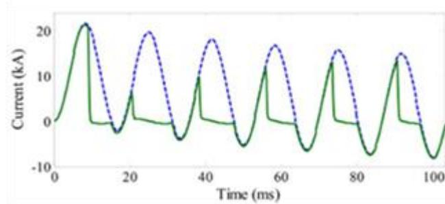
**Fig. 2.** Typical primary (dash line), scaled secondary (solid line), and CT magnetizing current (dash-dot line) of a saturated CT due to inrush current [9]
