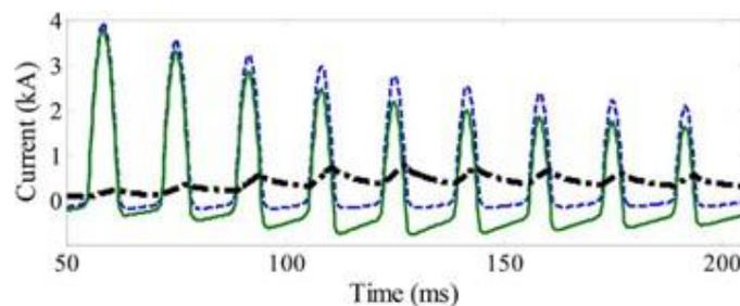
**Fig. 1.** Typical primary (dash line) and scaled secondary (solid line) of a saturated CT due to fault current [9]
