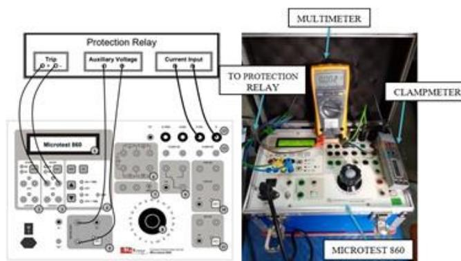
Fig. 7. Set-up the secondary current injection test
