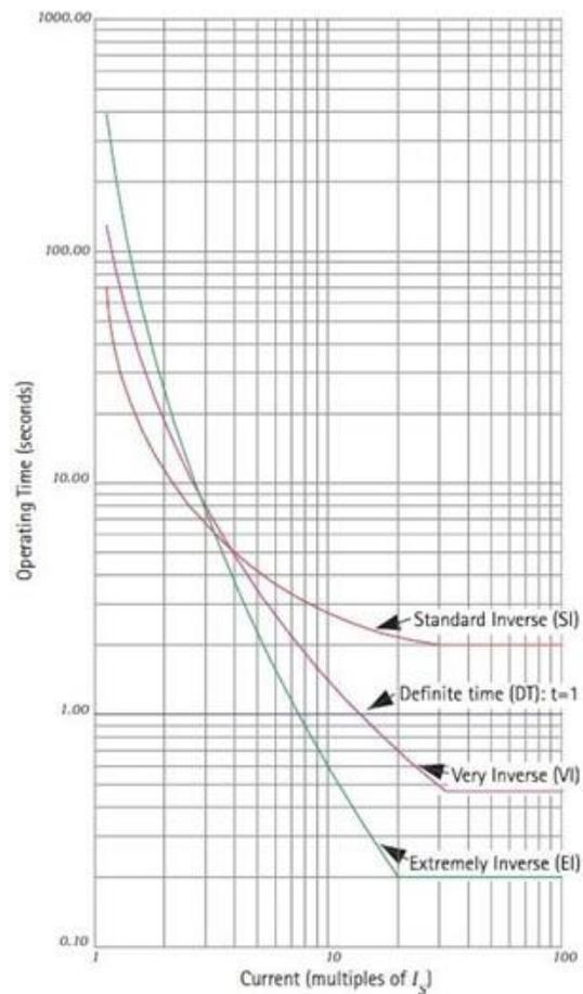
**Fig. 4.** IDMT relay characteristics of the overcurrent coordination
