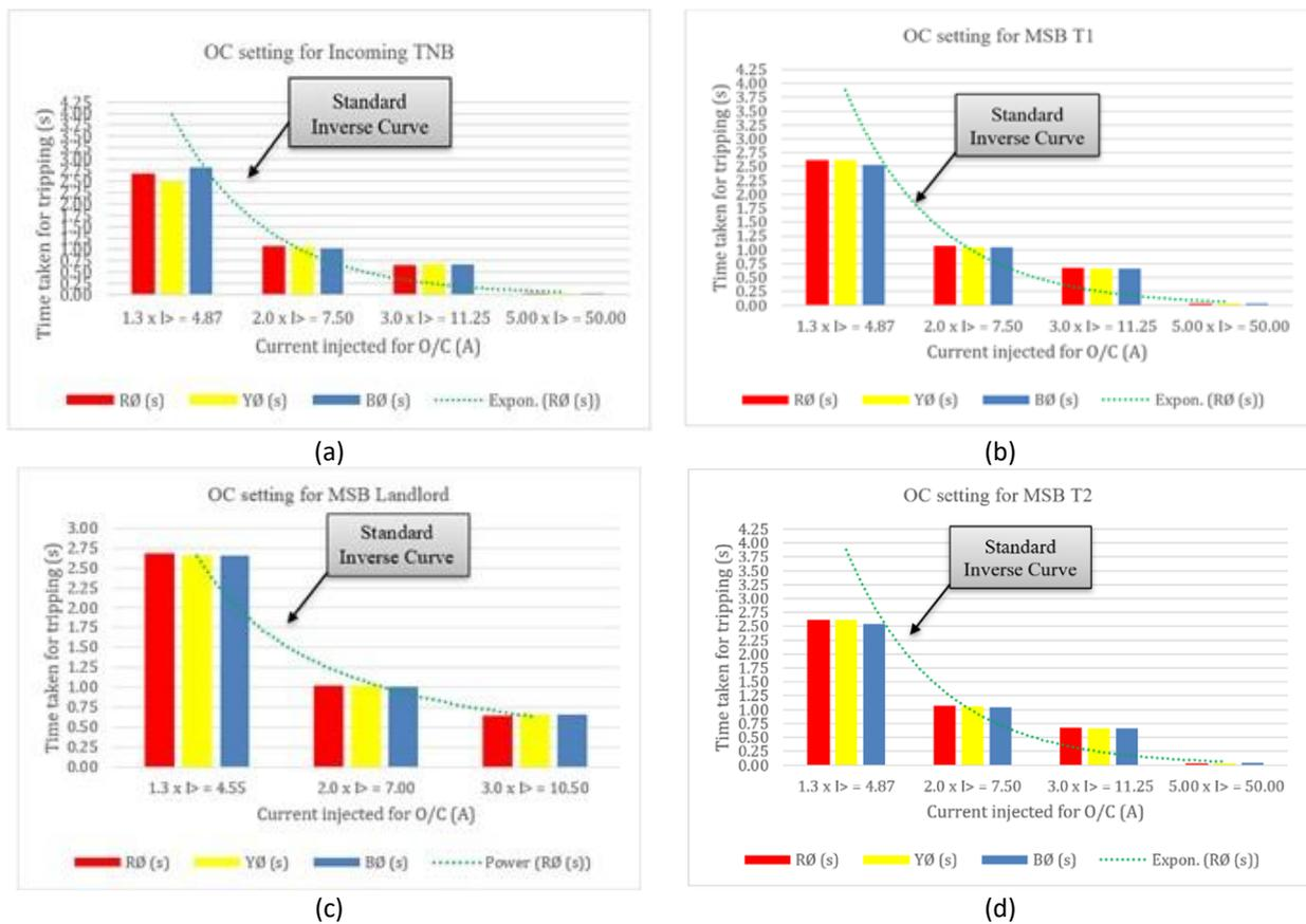
Fig. 8. The characteristics curve, (a) standard inverse (SI) for incoming TNB, (b) standard inverse (SI) for MSB T1, standard inverse (SI) for MSB T2, and (d) standard inverse (SI) for MSB Landlord
