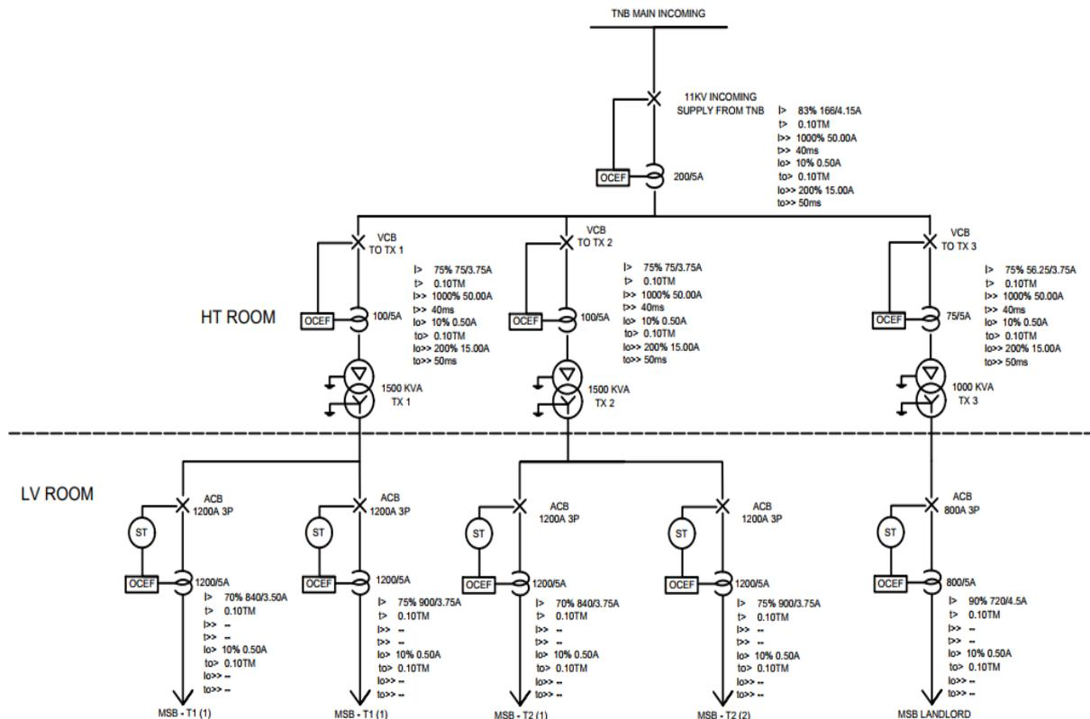
Fig. 6. Single-line diagram of 11kV commercial building in Malaysia
