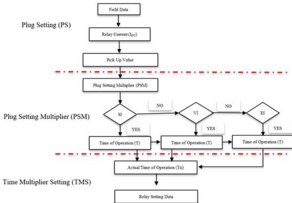
**Fig. 5.** Flow chart of the algorithm implemented in the overcurrent relay model [17]
