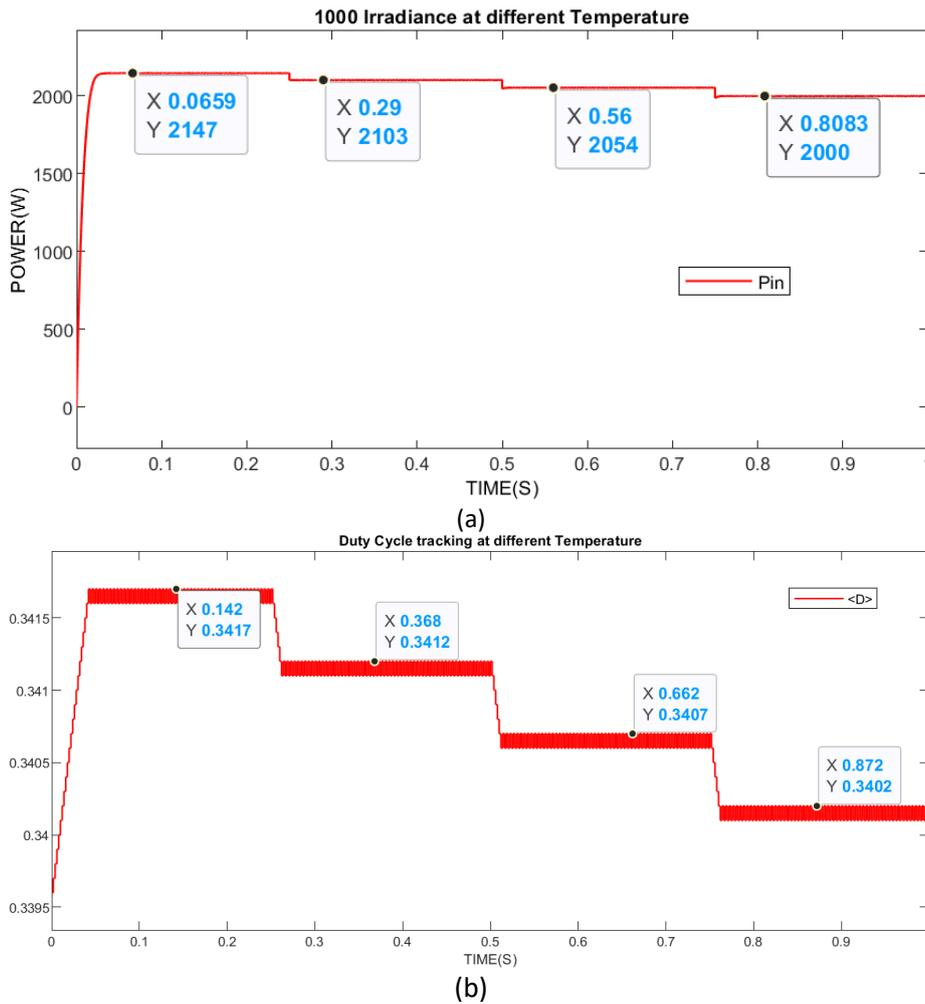
**Fig. 12.** 1000 W/m<sup>2</sup> Irradiance at 20°C, 25°C, 30°C, 35°C: (a) Maximum Power Point Tracking at Different Temperature, (b) Duty Cycle Perturbation for at Different Temperature.
