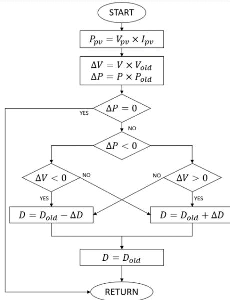
**Fig. 7.** The flowchart of P&O MPPT algorithm
