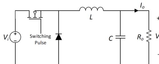
**Fig. 4.** The buck converter schematic diagram
