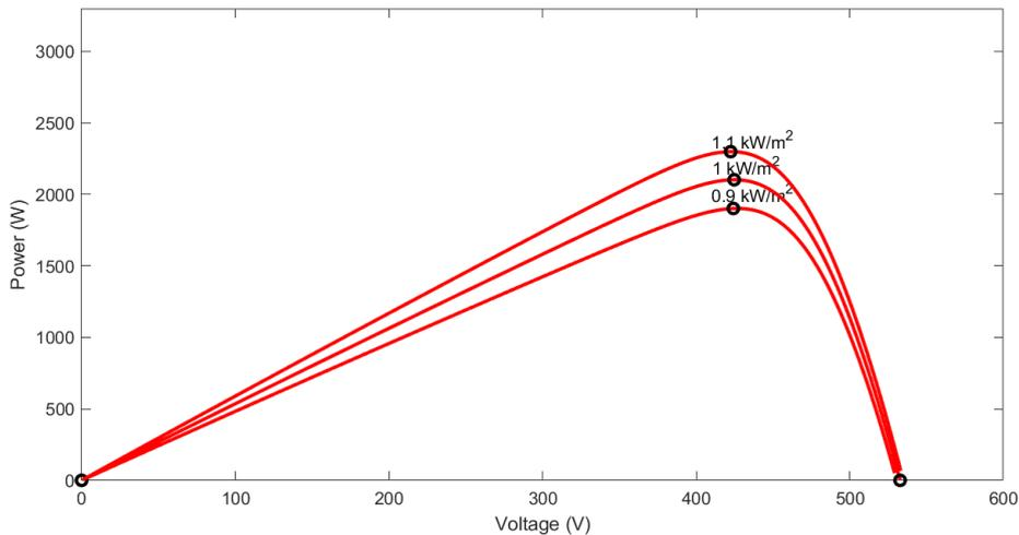
**Fig. 10.** PV-curve of different irradiance at 25°C
