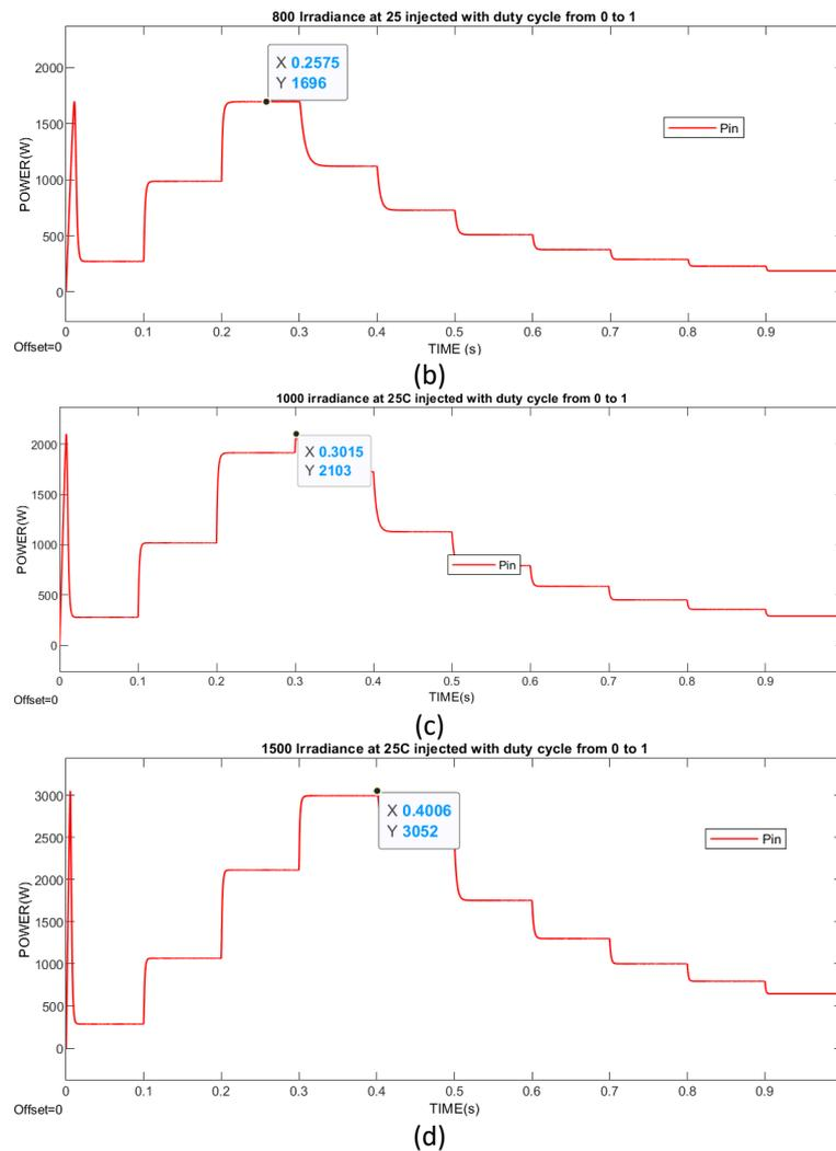
**Fig. 9.** MPP of Irradiance at 25°C with Duty Cycle from 0 to 1: (a) 500 W/m<sup>2</sup>, (b) 800 W/m<sup>2</sup>, (c) 1000 W/m<sup>2</sup>, (d) 1500 W/m<sup>2</sup>
