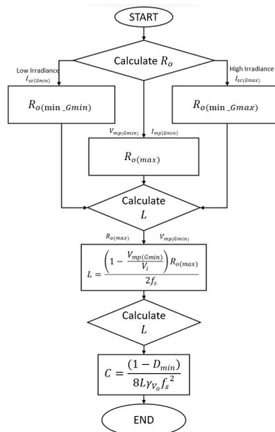
**Fig. 6.** The flowchart of the MPPT buck converter
