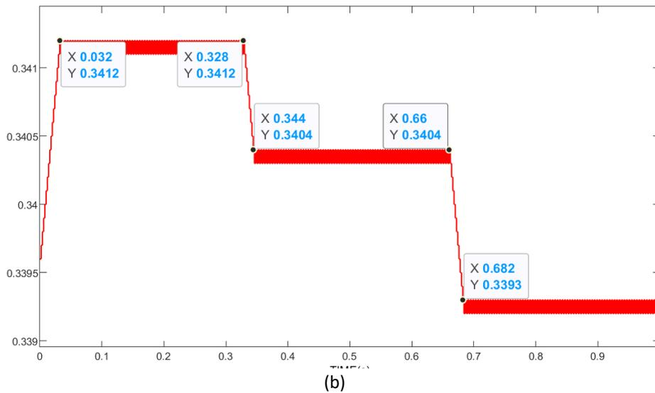
**Fig. 11.** 1100 W/m<sup>2</sup>, 1000 W/m<sup>2</sup>, 900 W/m<sup>2</sup> Irradiance at 25°C: (a) Maximum Power Point Tracking at Different Irradiance, (b) Duty Cycle Perturbation at Different Irradiance
