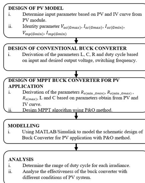
Fig. 1. The overall flow of methodology
