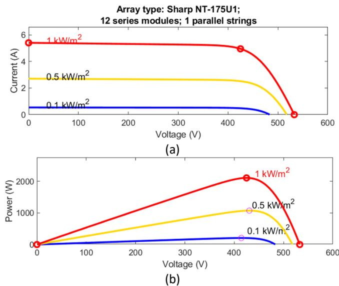
**Fig. 3.** The characteristics curve produced by the PV model (a) The current-voltage (I-V) curve (b) The power-voltage (P-V) curve
