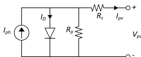
Fig. 2. Single diode mode schematic
