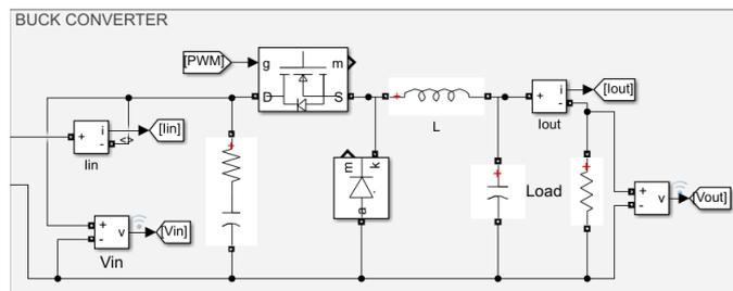
Fig. 5. The block of buck converter in MATLAB/Simulink
