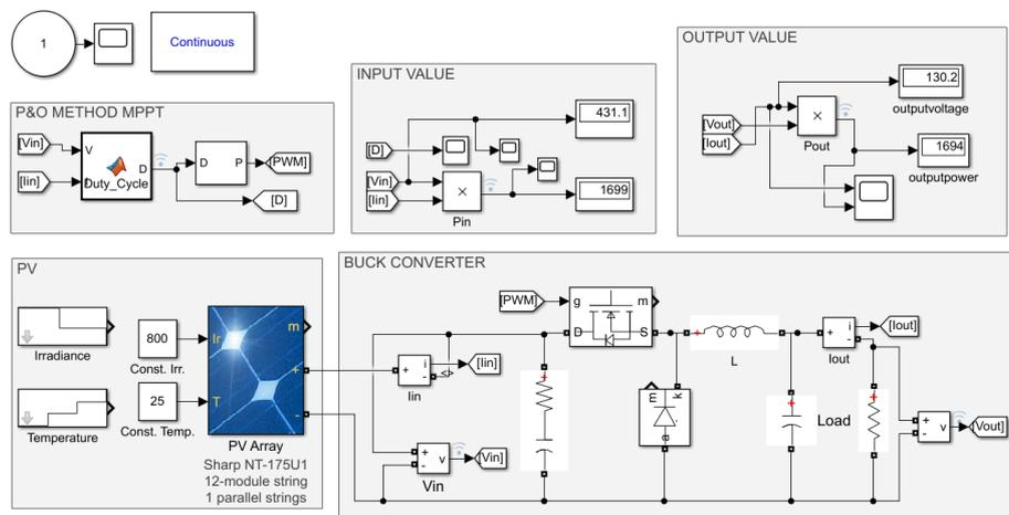
Fig. 8. The block of MPPT buck converter
