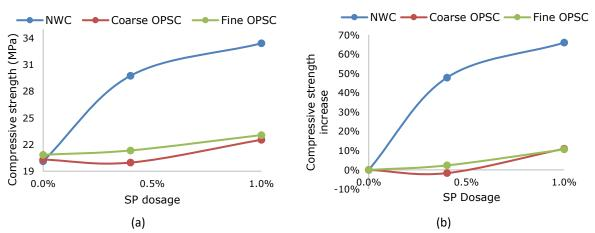
Fig. 8. Influence on compressive strength with addition of SP dosage
