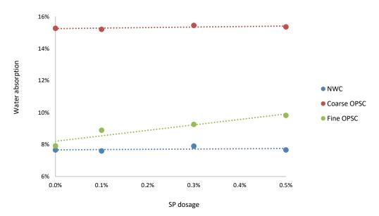
Fig. 6. Influence on water absorption with increase of SP dosage
