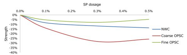
Fig. 3. Influence on 7 days compressive strength with increase of SP dosage
