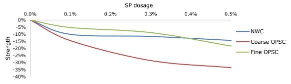
Fig. 4. Influence on 28 days compressive strength with increase of SP dosage
