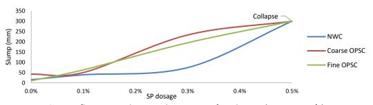
Fig. 2. Influence on slump with increase of SP dosage (constant w/c)
