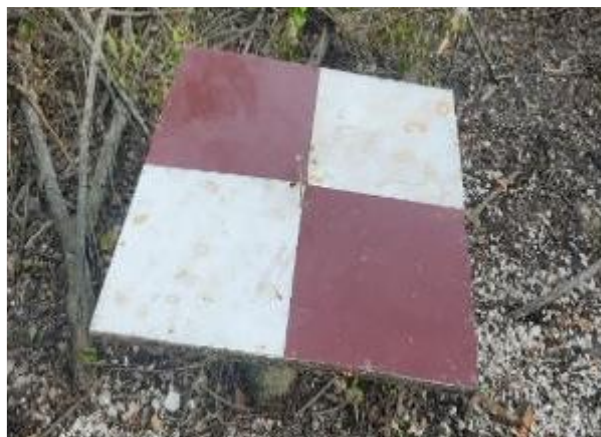
Fig. 2. Ground control point (GCP)
