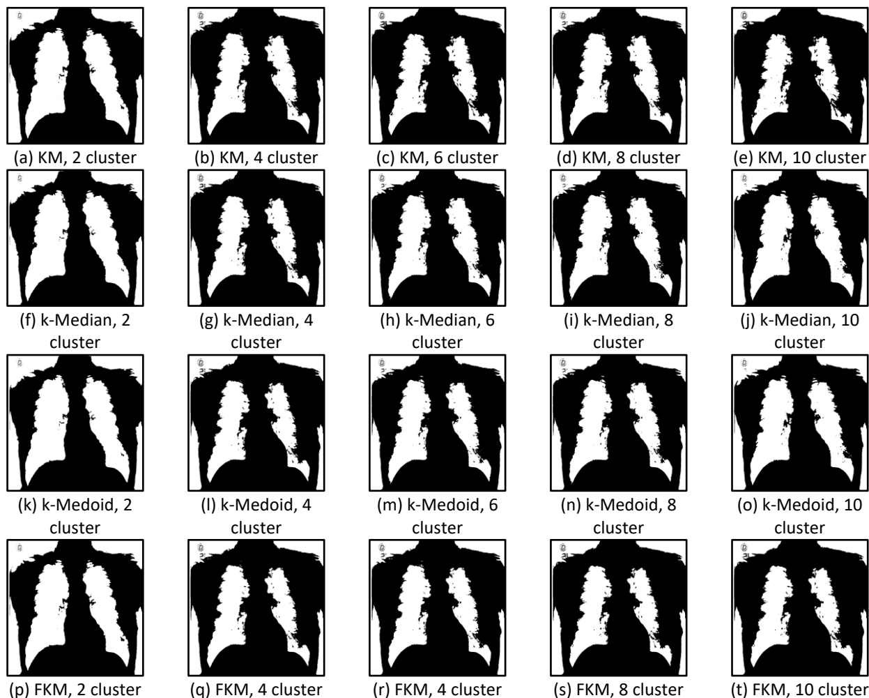
Fig. 3. Comparison of the k-means, k-medians, k-medoids and fast k-means with 2, 4, 6, 8, 10 number of clusters with COVID-19 infected lung image. The foreground filter from the number of clusters is unified at 50%
