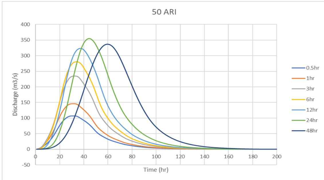
**Fig. 3.** HEC-HMS hydrograph for 30 minutes until 2 days duration (50 ARI)
