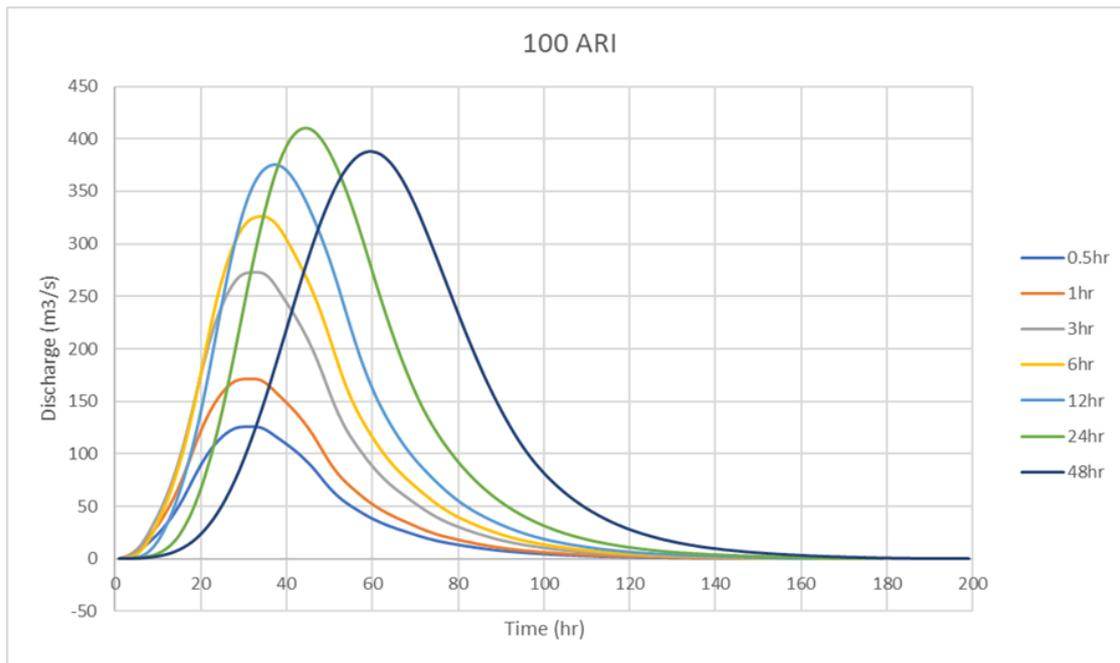
**Fig. 4.** HEC-HMS hydrograph for 30 minutes until 2 days duration (100 ARI)
