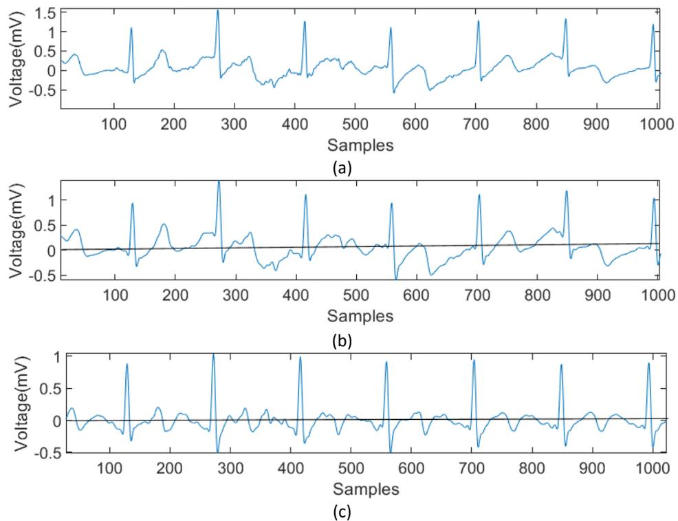
**Fig. 4.** ECG Signal Through Pre-processing Process (a) Raw ECG, (b) Filtered ECG, (c) Detrend ECG
