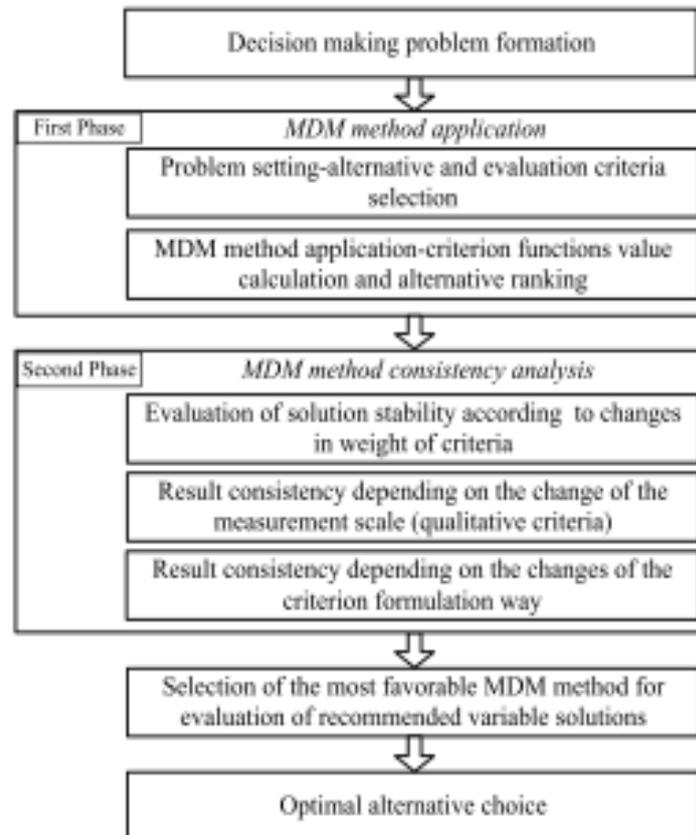
Fig. 2. Model of result consistency evaluation in MCDM
