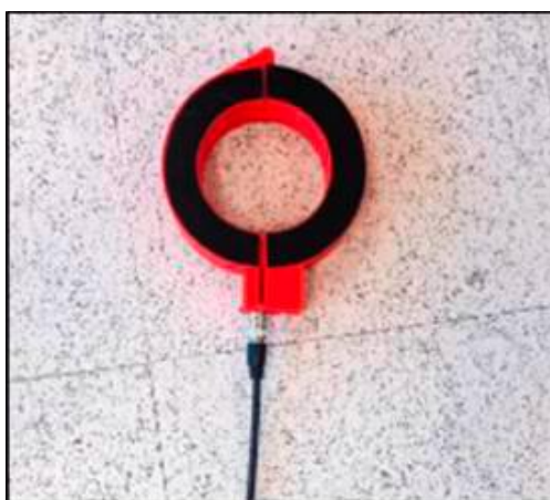
Fig. 1. Rogowski Coil sensor for partial discharge detection
