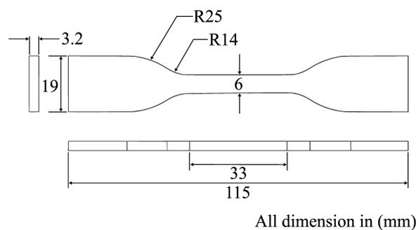
**Fig. 1.** Sample design according to ASTM D638-IV
