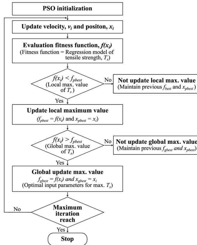
Fig. 4. PSO algorithm for optimization of tensile strength
