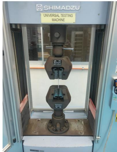
**Fig. 2.** Universal testing machine
