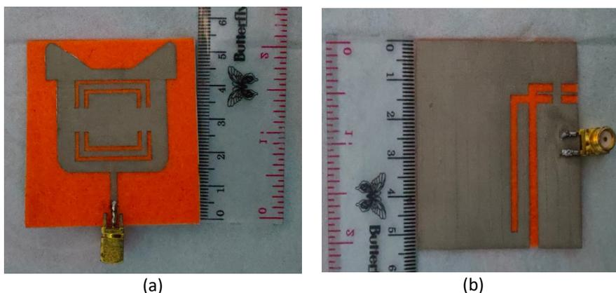
**Fig. 2.** Fabricated textile antenna (a) Front view and (b) Back view
