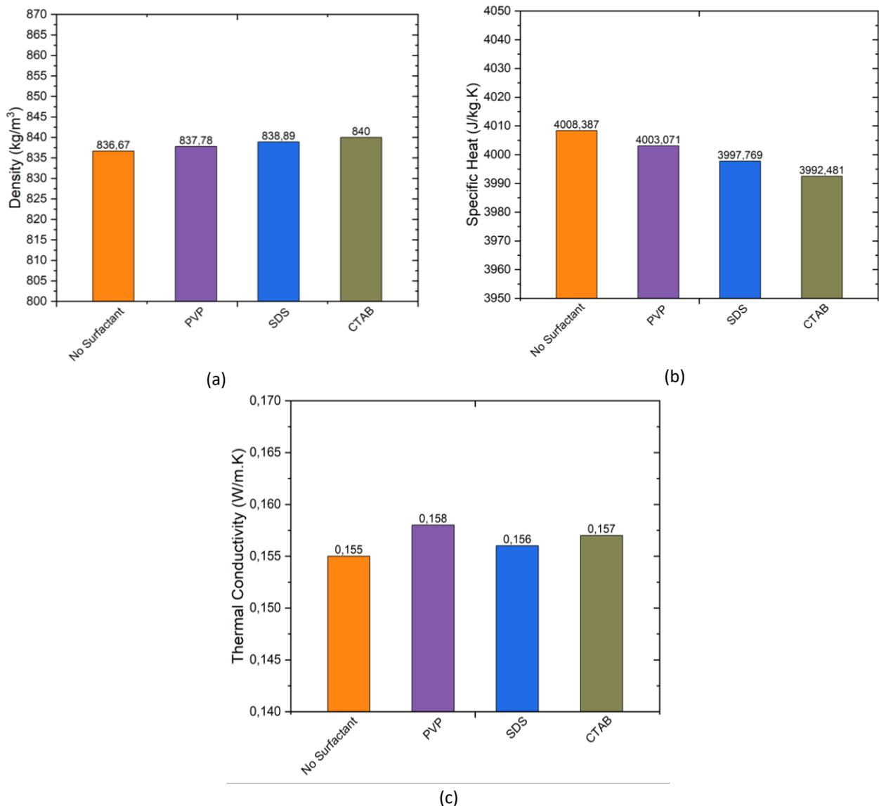
**Fig. 5.** Graphics of (a) Density, (b) Specific heat, and (c) Thermal conductivity of VCO-GNP Bio-Nanofluid
