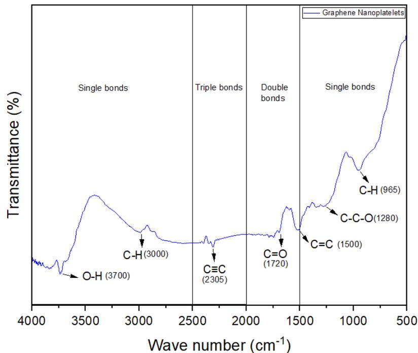
Fig. 4. FTIR results of graphene nanoplatelets nanoparticle
