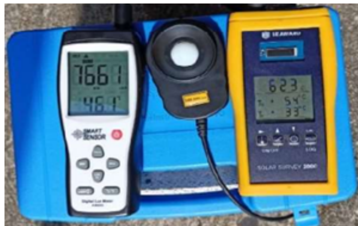
Fig. 3. Measurement of lux meter and solar survey
