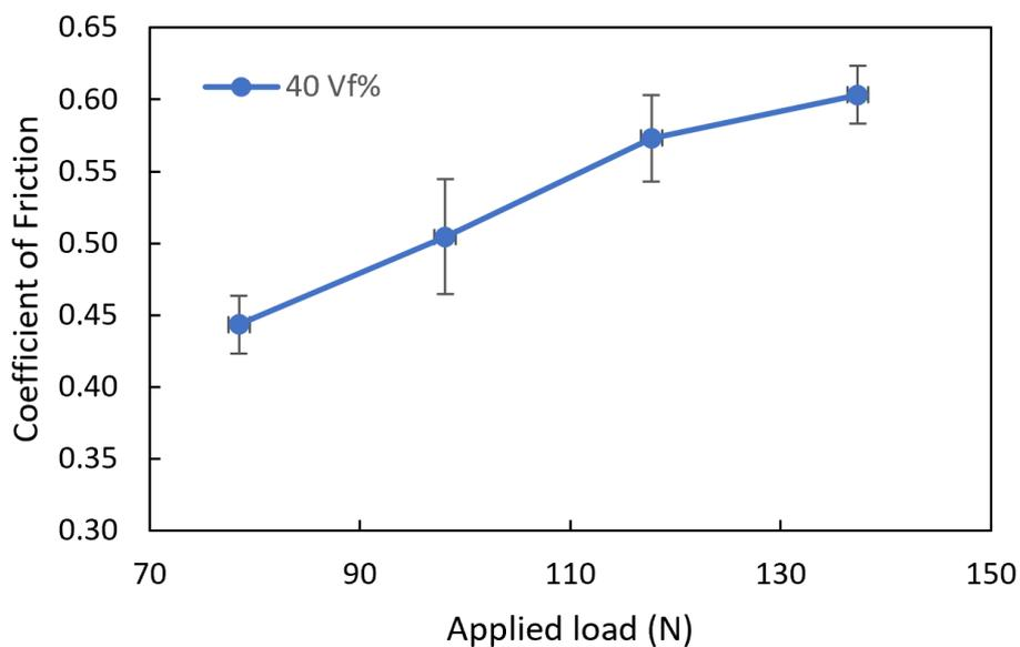
Fig. 3. Coefficient of friction vs applied load
