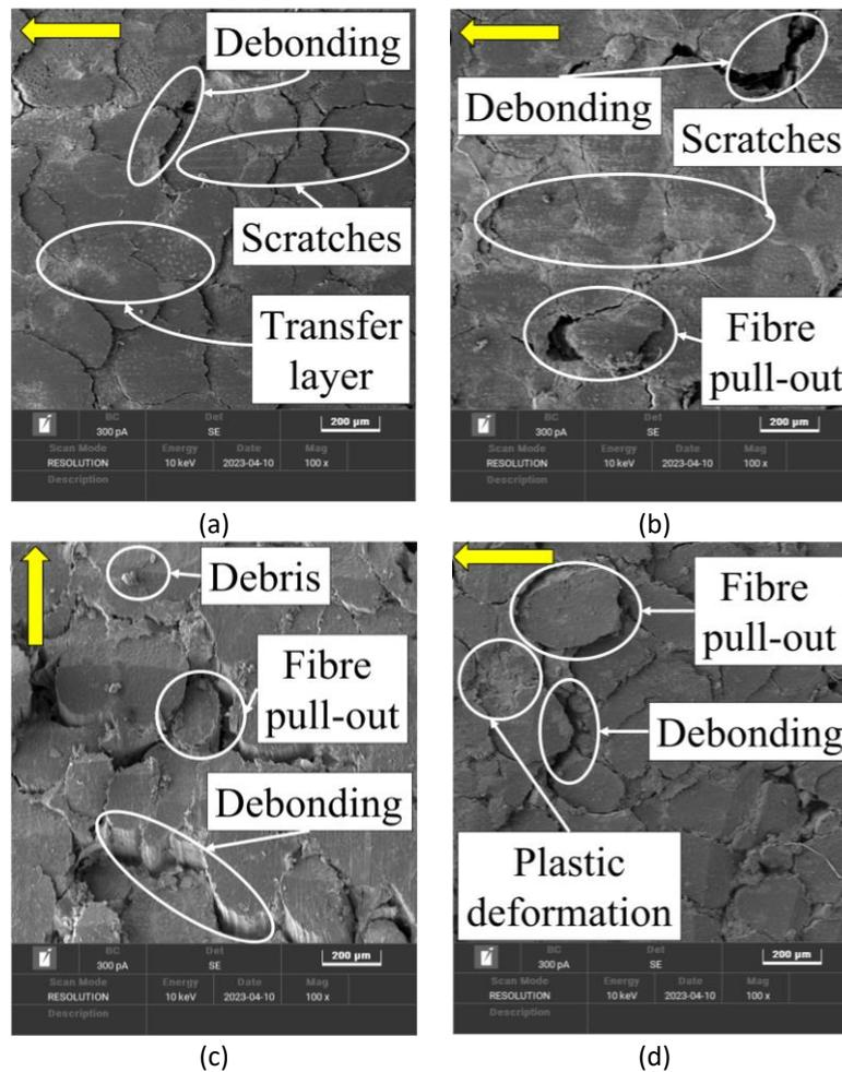
**Fig. 5.** Scanning electron microscopy (SEM) images of normal orientation *Furcraea Foetida* fibre reinforced epoxy composite under applied loads of (a) 80N, (b) 100N, (c) 120N and (d) 140N. The yellow arrow represents sliding direction
