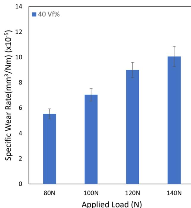
Fig. 4. Specific wear rate vs applied load
