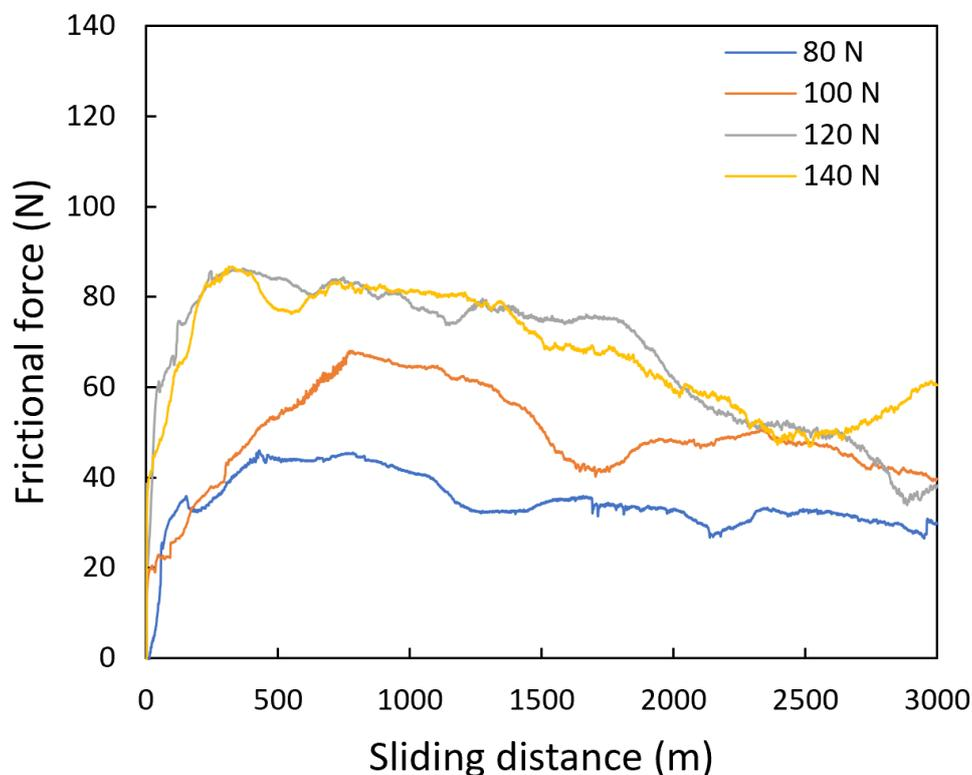
**Fig. 2.** Frictional force vs sliding distance for normal orientation with 40Vf%
