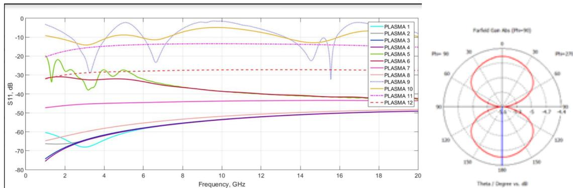
**Fig. 2.** Result of return loss (left) and radiation pattern (right) for 1D-split ring structure
