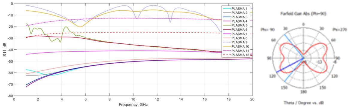
**Fig. 4.** Results of return loss (left) and radiation pattern (right) for omega structure
