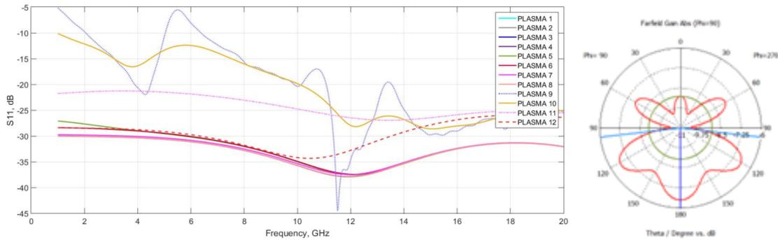
**Fig. 3.** Results of return loss (left) and radiation pattern (right) for symmetrical ring structure
