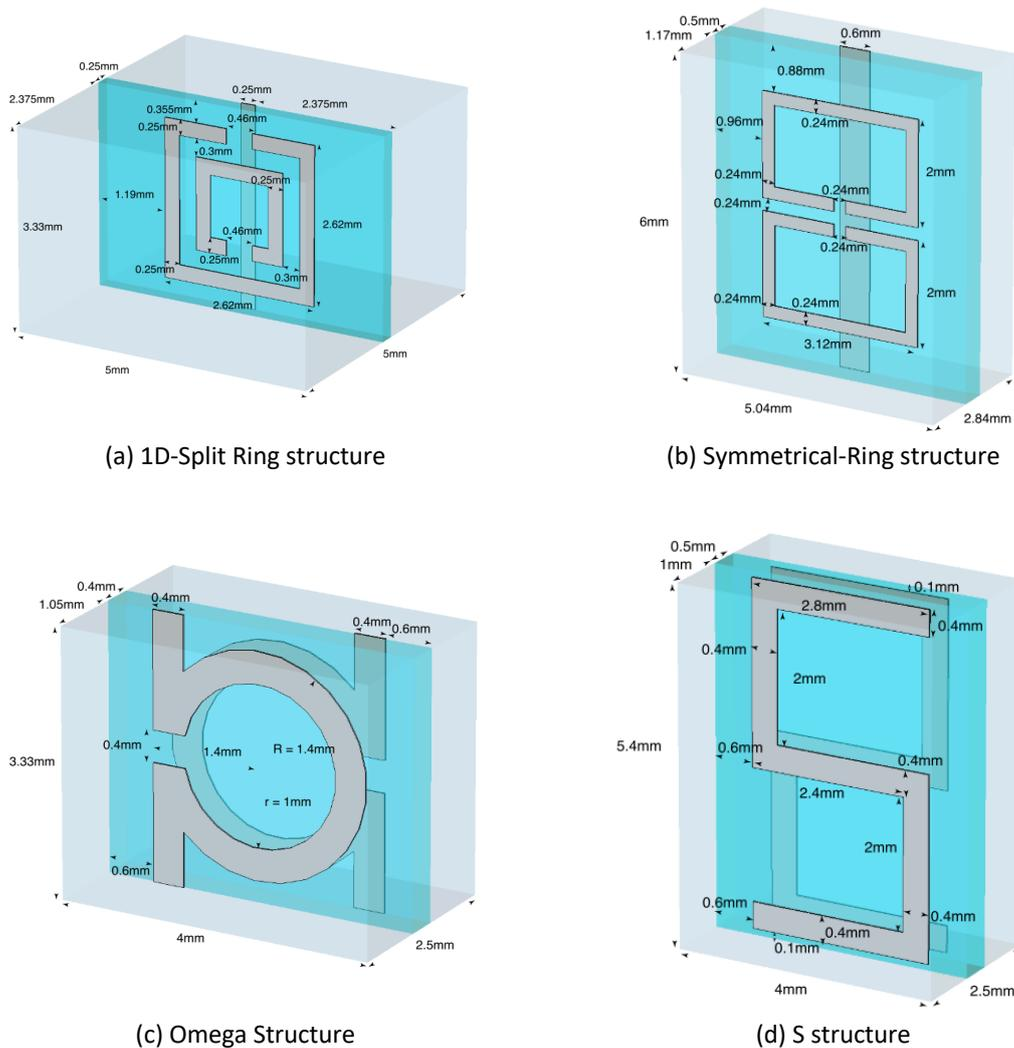
**Fig. 1.** Metamaterial structures used in this study, composing 4 types of unit cell structures i.e., 1D-Split Ring Resonator, Symmetrical Ring, Omega and S structures [17]
