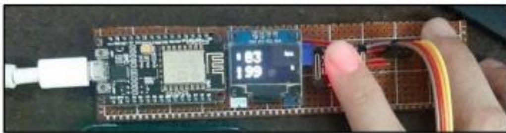
Fig. 3. The parameters shown on OLED when data measure using Vital Sign Sensors
