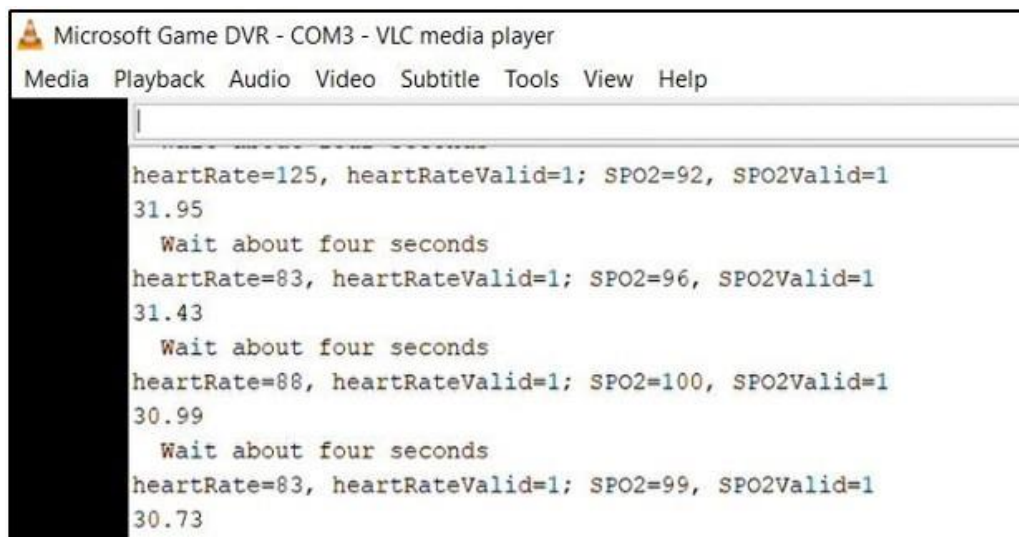
Fig. 4. The results displayed in serial monitor when system start to measure the Vital Sign Data
