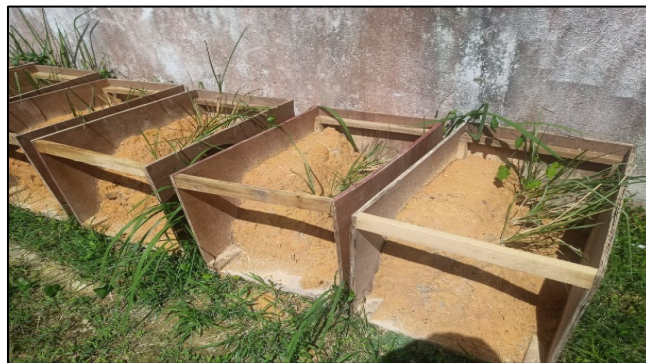
Fig. 1. Physical root-soil modelling with varies of slope gradients
