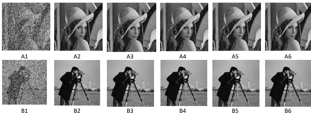
Fig. 4. Lena and Camera images corrupted by 60 % salt-and-pepper noise: (A1, B1), the restored images using SFA: (A2, B2), LS: (A3, B3), HS: (A4, B4), DY: (A5, B5), and RMIL: (A6, B6)
