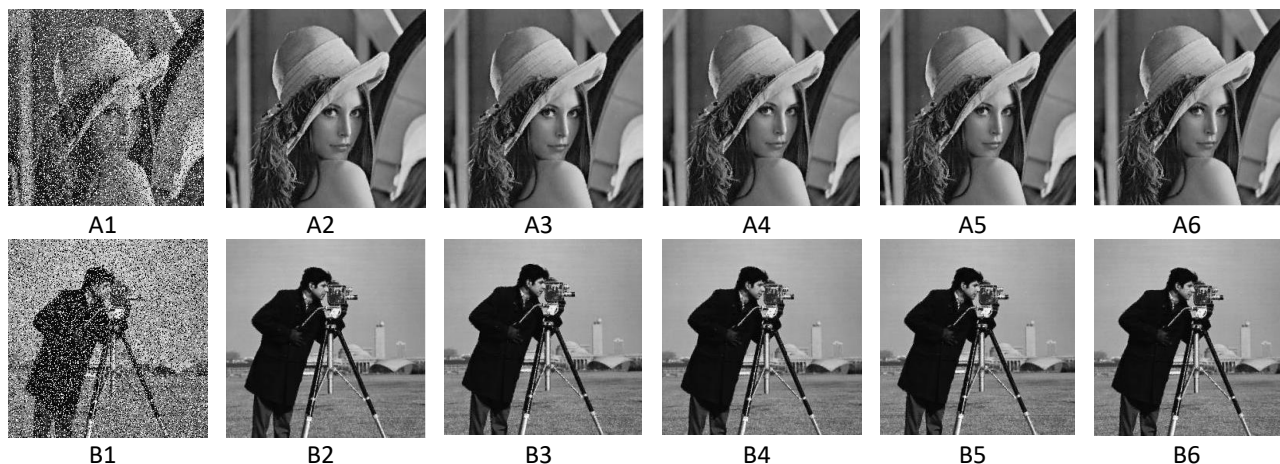
Fig. 3. Lena and Camera images corrupted by 30 % salt-and-pepper noise: (A1, B1), the restored images using SFA: (A2, B2), LS: (A3, B3), HS: (A4, B4), DY: (A5, B5), and RMIL: (A6, B6)
