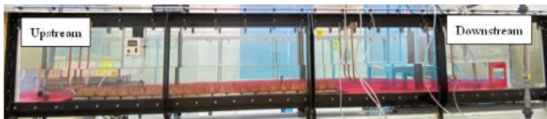
Fig. 4. Concentration of red dye tracer during light rainfall conditions with morphology effect (represent by artificial roughened bed section)
