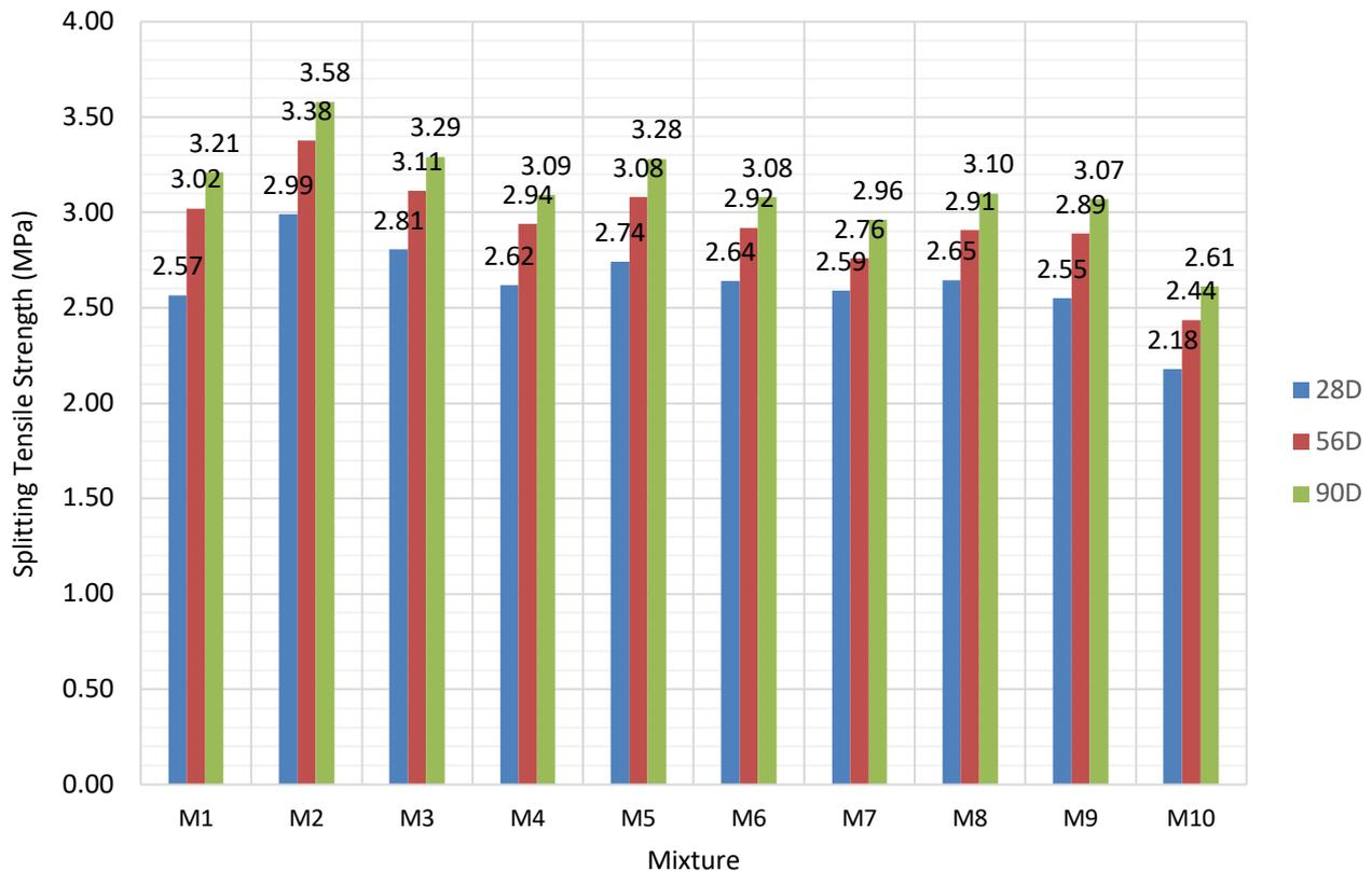
Fig. 8. Splitting tensile strength test
