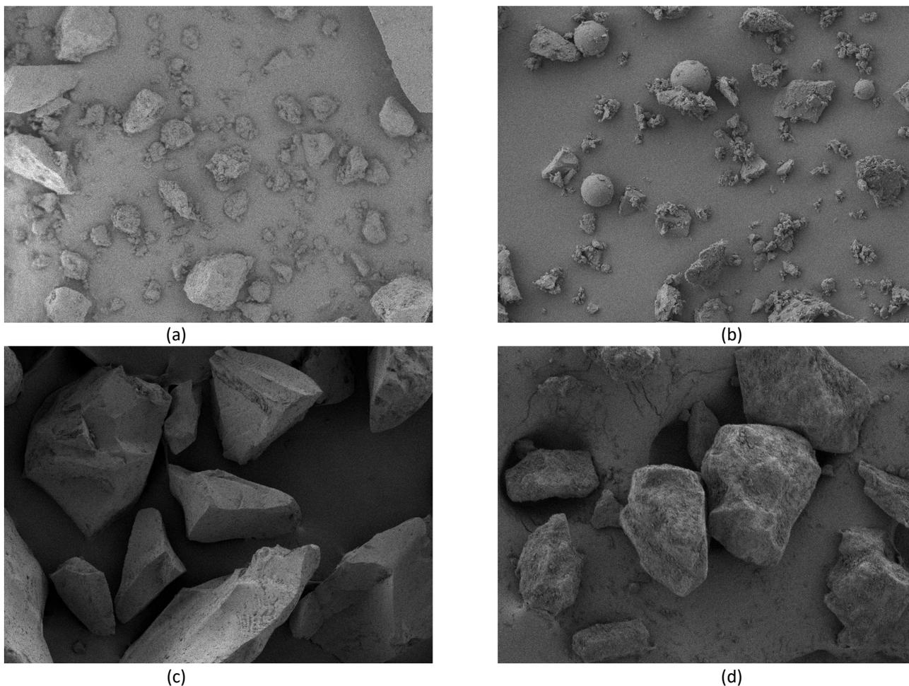
**Fig. 3.** The morphology by FE-SEM of (a) uCBA with 1000x magnify, (b) OPC with 1000x magnify, (c) SG with 500x magnify, and (d) fine aggregate with 500x magnify
