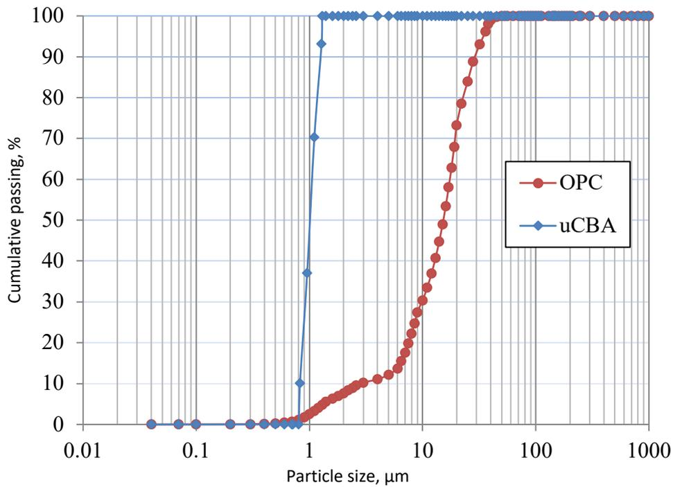
**Fig. 4.** Particle size distribution by cumulative passing of uCBA and OPC
