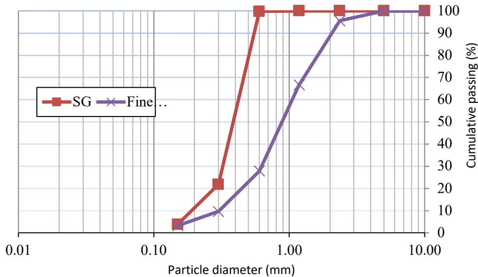
**Fig. 5.** Sieve analysis of SG and fine aggregate
