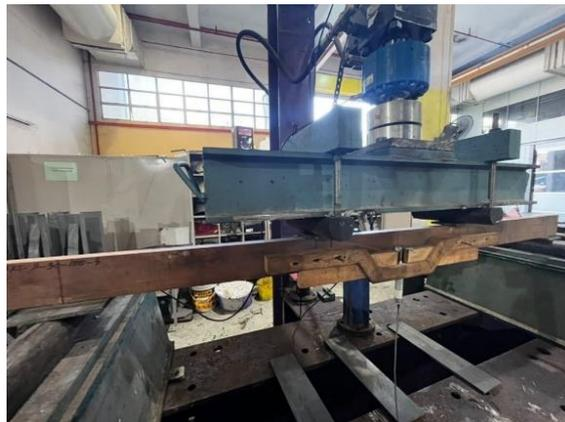
**Fig. 2.** Set up machine for bending test
