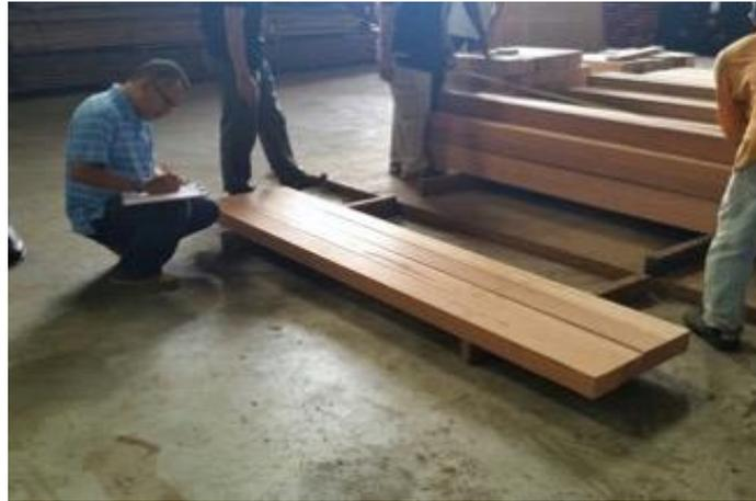
**Fig. 1.** Timber specimens graded by MTIB certified graders
