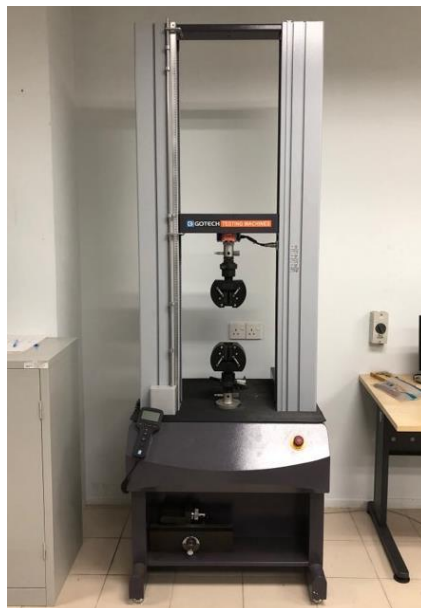
Fig. 4. GoTech universal testing machine AI-7000L used for the compression loading test
