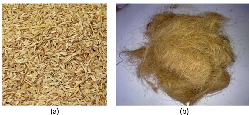
Fig. 1. Raw materials: (a) rice husk (b) coconut fibre
