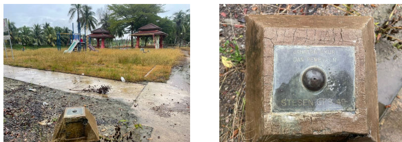
Fig. 7. JUPEM GPS Station (GPS Station 49)
