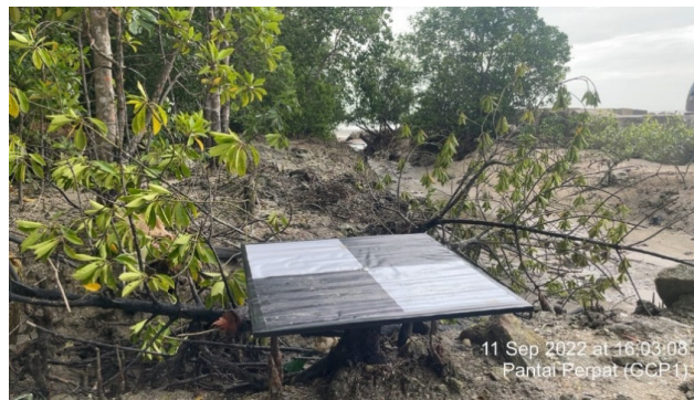
Fig. 6. GCP boards are placed on mangrove trees
