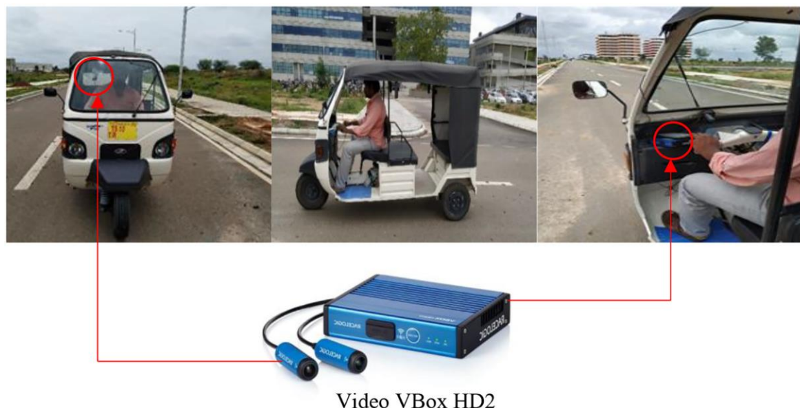
Fig. 3. Instrumented test vehicle used for the study (Source: Chandrashekar et al. ,) [41]
