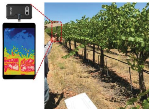
Fig. 6. CWSI instrument: thermal sensor attached to tablet proving thermal image [21]
