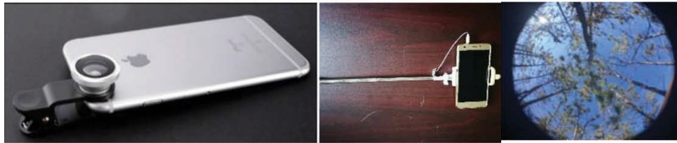
Fig. 3. LAI-Mobile instrument: (a) mobile phone equipped with spherical lens; (b) mobile phone fixed with selfie stick; (c) an example fisheye image acquired by LAI-Mobile [38]
