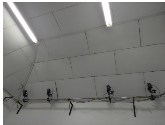
Fig. 4. A total of 8 camera of Motion Capture have been used to capture the movement
