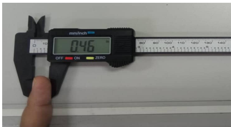
Fig. 5. Finger Circumference Measurement with A Digital Caliper
