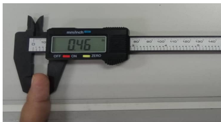
Fig. 5. Finger Circumference Measurement with A Digital Caliper
