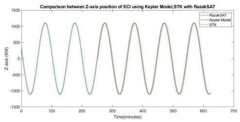
**Fig. 8.** Comparison of ECI around X, Y, Z-axes using Keplerian orbit model, STK, and RazakSAT
