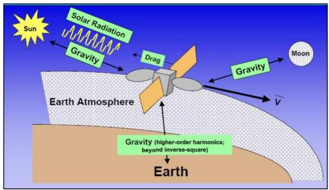
Fig. 2. Disturbances forces effecting orbit [11]
