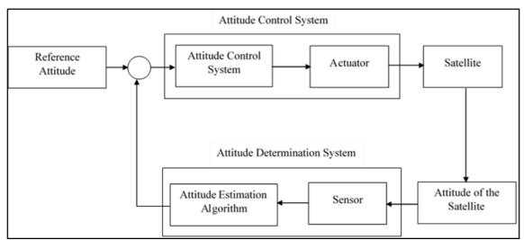
Fig. 1. Block diagram of an ADCS
