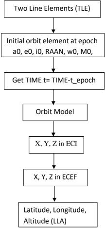
Fig. 7. Process of orbit model Kepler
