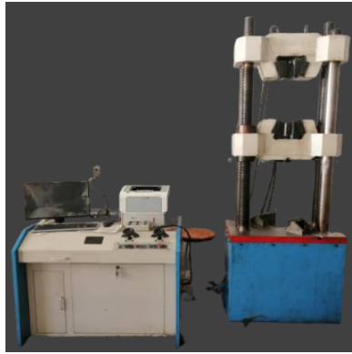
Fig. 2. The apparatus used for conducting tensile testing
