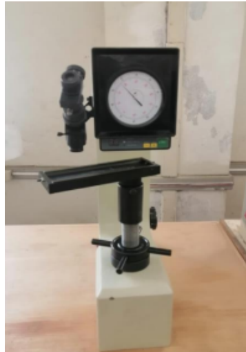
Fig. 5. Machine for measuring microhardness
