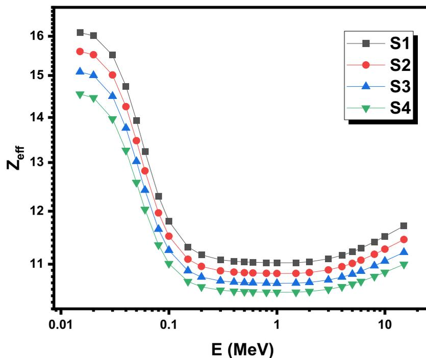
**Fig. 2.** The effective atomic number for the CaO–Al<sub>2</sub>O<sub>3</sub>–SiO<sub>2</sub> glass systems with constant amount of SiO<sub>2</sub> (60 mol%)
