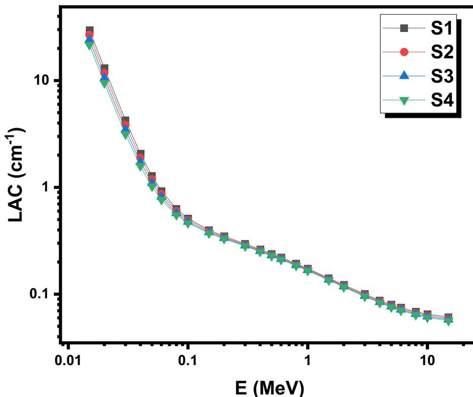
**Fig. 1.** The linear attenuation coefficient for the CaO–Al<sub>2</sub>O<sub>3</sub>–SiO<sub>2</sub> glass systems with constant amount of SiO<sub>2</sub> (60 mol%)
