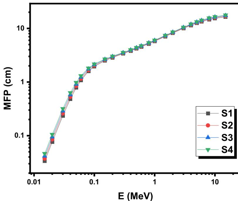
Fig. 5. The mean free path for the selected glasses at 0.1, 0.5 and 1 MeV
