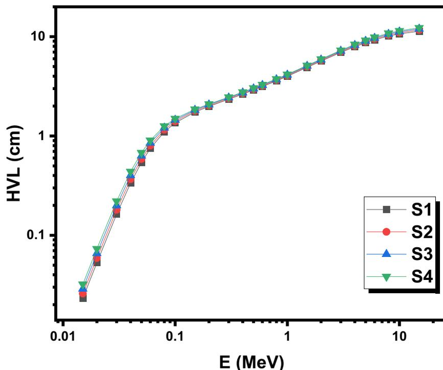
**Fig. 3.** The half value layer for the CaO–Al<sub>2</sub>O<sub>3</sub>–SiO<sub>2</sub> glass systems with constant amount of SiO<sub>2</sub> (60 mol%)
