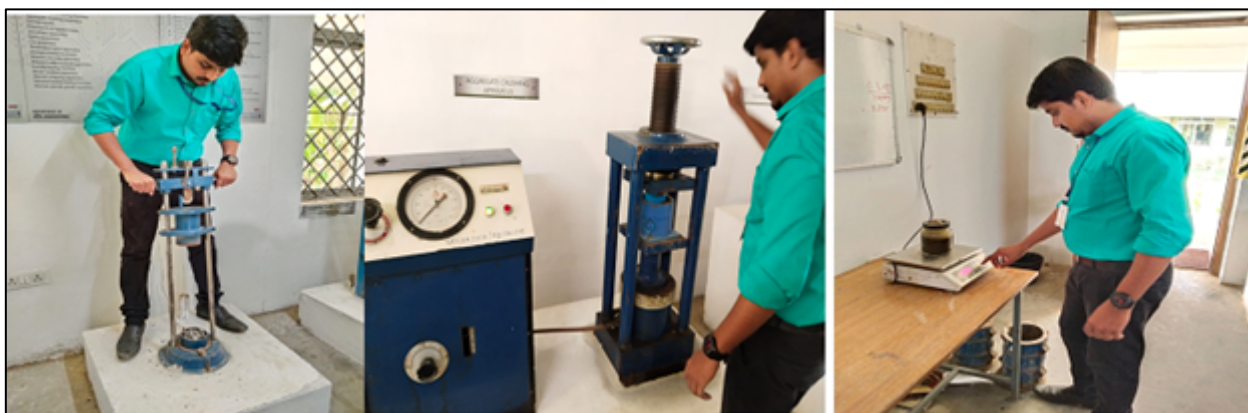
Fig. 7. (a) Aggregate Impact Value Test Conducted (b) Aggregate Crushing Strength Test Conducted (c) Aggregate Water Absorption Test Conducted
