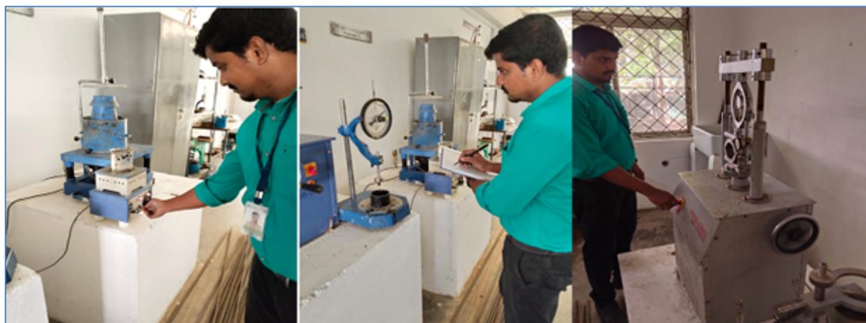
Fig. 9. (a) Bitumen Softening Point Value (b) Bitumen Penetration Value (c) Marshal Stability Test Conducted on Bitumen
