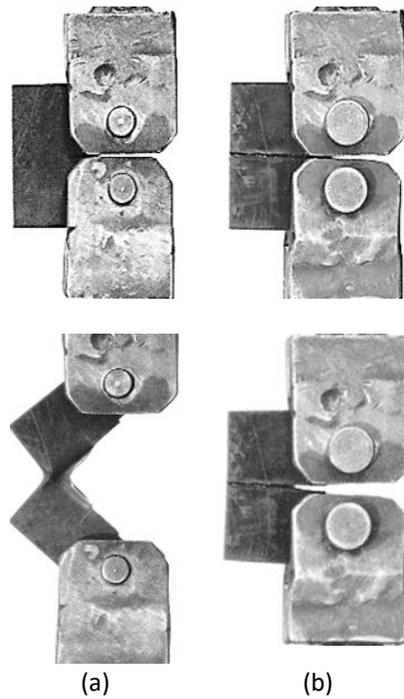
**Fig. 7.** Experiment Fracture Toughness (a) without side grooves, (b) with side grooves
