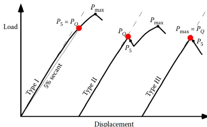
Fig. 5. PQ value on the graph of the load
