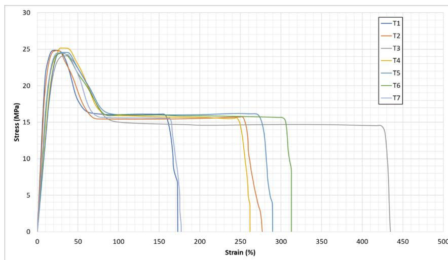
Fig. 6. Stress and Strain curve of HDPE
