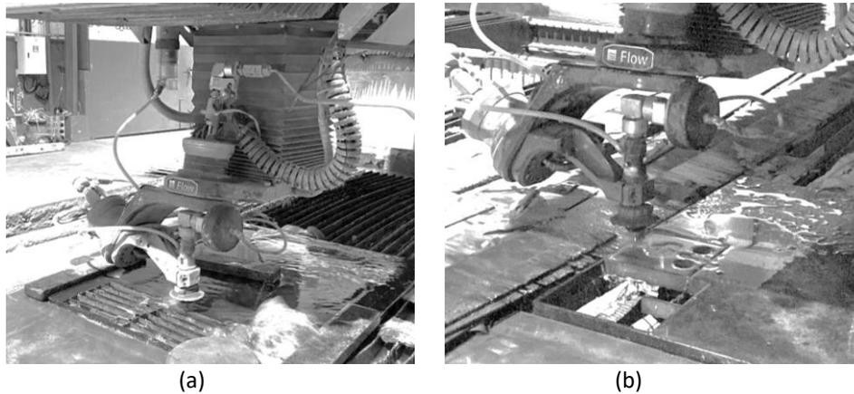
**Fig. 2.** Cutting specimen processing; (a) Tensile, (b) compact tension
