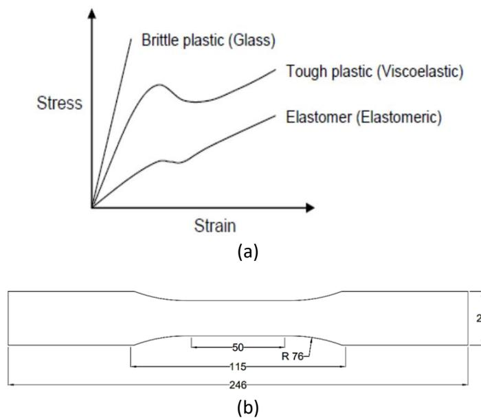
**Fig. 1.** Polymer Materials; (a) stress-strain diagram, (b) detailed specimen dimensions [3]
