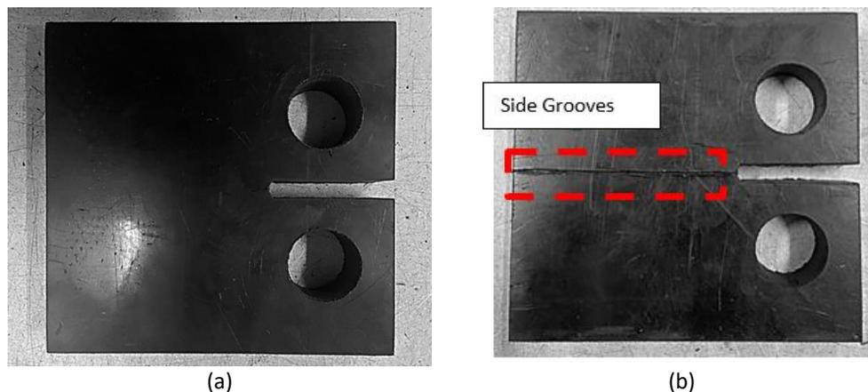
**Fig. 4.** Variation of compact tension specimen models: (a) no crack, and (b) side grooves
