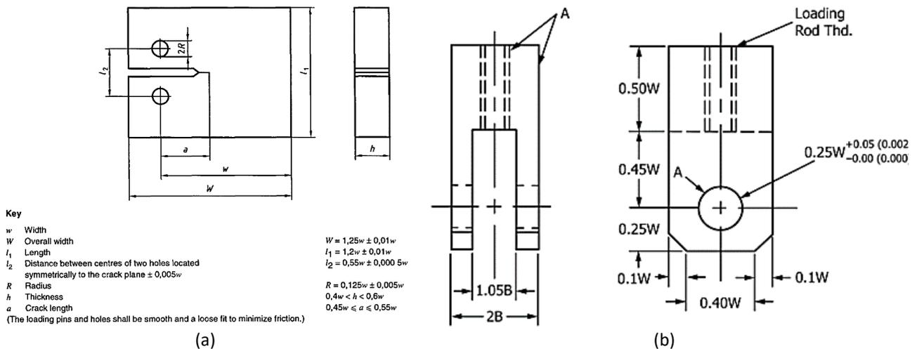
**Fig. 3.** (a) Toughness Test Specimen and (b) Compact Tension Specimen Grip Design (ISO-13586 2018)
