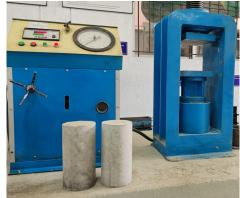
Fig. 7. Coired Concrete - Cylinder Specimens
