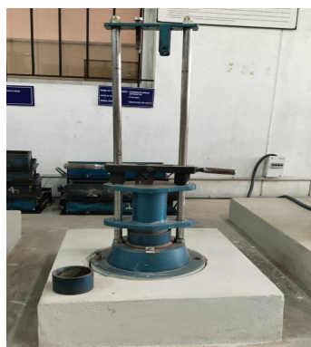
Fig. 3. The drop weight impact machine is shown in a systematic diagram
