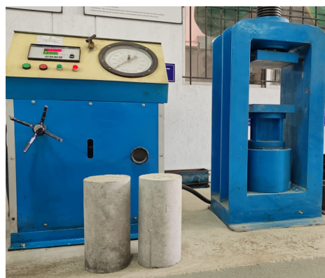
Fig. 7. Coired Concrete - Cylinder Specimens
