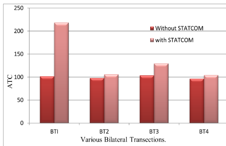
Fig. 9. Comparison of ATC with/without STATCOM for all Bilateral Transactions under generator 3 out of the network
