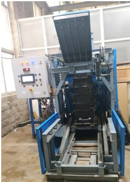
Fig. 2. Roller compactor and rut analyzer (RCRA) equipment
