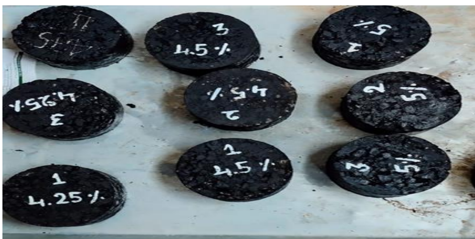
Fig. 1. Marshall specimens at different binder content
