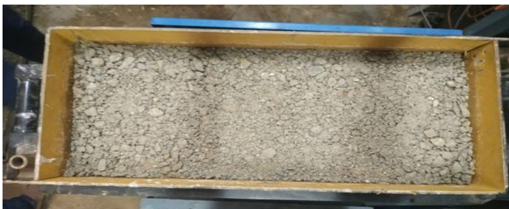
Fig. 4. Casting of base course (WMM) layer
