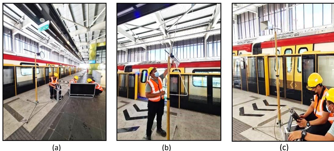
Fig. 3. Example of measurement set-up using (a) Loop antenna (b) Tri-log antenna (c) Horn antenna
