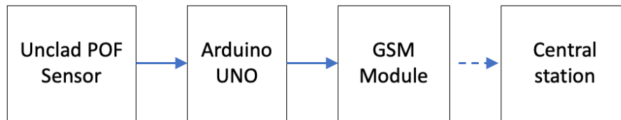
Fig. 4. Monitoring system block diagram
